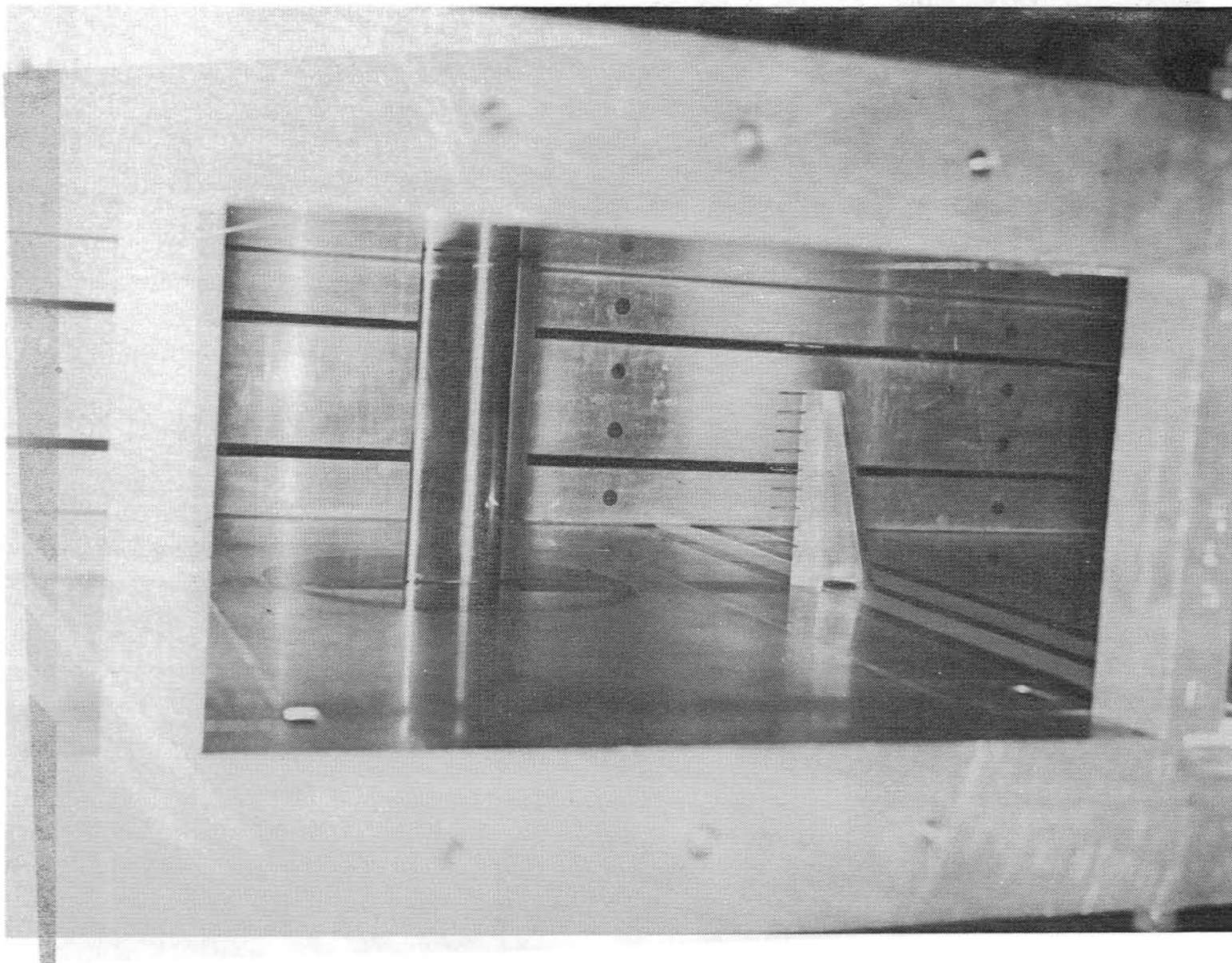
Figure 5.— 7.62 cm chord CAST 10-2/DOA 2 model installed in two dimensional test section.
