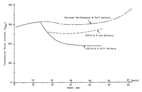
Figure 3.4.4-1 AC Motor Current
