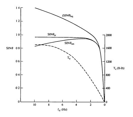
Figure 3.5.3-1 Induction Motor Angle and Torque as Function of Slip Frequency
