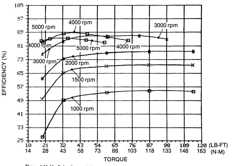
Figure 4.11-10 Drive System Efficiency in Regenerative Braking Note: Speed and torque are at the gear box shaft after the 2.923:1 reduction.
