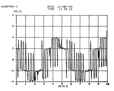
Figure 4.7-4 Motor Line-to-Neutral Voltage in PWM Regenerative Braking Note: Voltage (vertical) scale factor is 20 volts/volt, time (horizontal) scale is in milliseconds.
