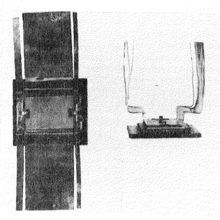
Figure 3.8.3-1 Top and Side Views of the Darlington Transistor in Subscrete Form
