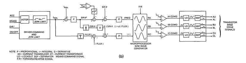
Figure 3.6-3 Control Function Block Diagram
