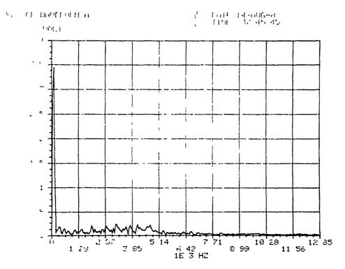
Figure 4.6-2 Frequency Spectrum of PWM Motoring Current Note: Current (vertical) scale factor is 80 amps/volt, frequency (horizontal) scale is in kilohertz.
