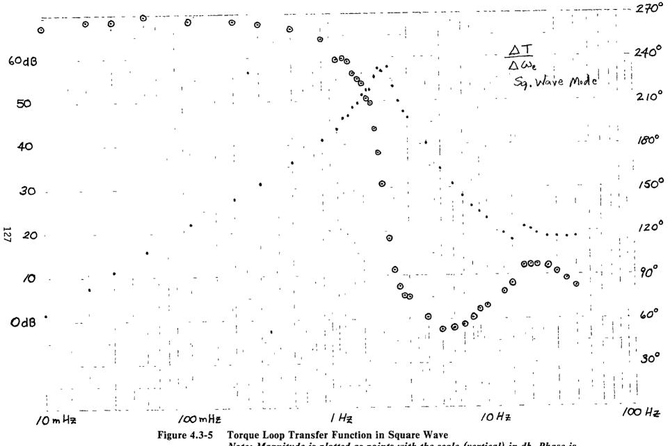
Note: Magnitude is plotted as points with the scale (vertical) in db, Phase is plotted as circled points with the scale (vertical) in degrees, Frequency is the horizontal scale.
