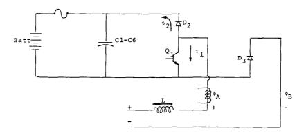
Figure 3.11.4-1 Active Components for Positive Half Cycle
