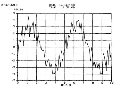
Figure 4.7-3 Motor Current in PWM Motoring Note: Current (vertical) scale factor is 80 amps/volt, time (horizontal) scale is in milliseconds.
