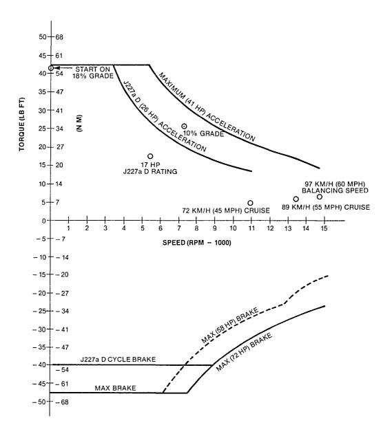
Figure 3.2.3-1 Motor Torque and Speed Requirement
