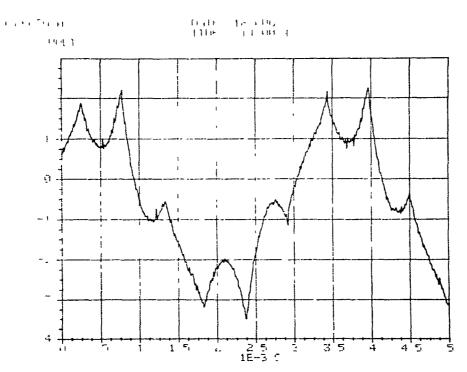
Figure 4.6-3 Motor Current in Square Wave Motoring Note: Current (vertical) scale factor is 80 amps/volt, time (horizontal) scale is in milliseconds. Waveform is slightly offset from zero.
