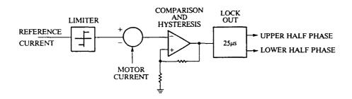
Figure 3.5.2-3 Current Control Circuit for One Phase
