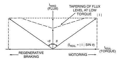
Figure 3.6.2.1-1 Imaginary and Real Components of Current
