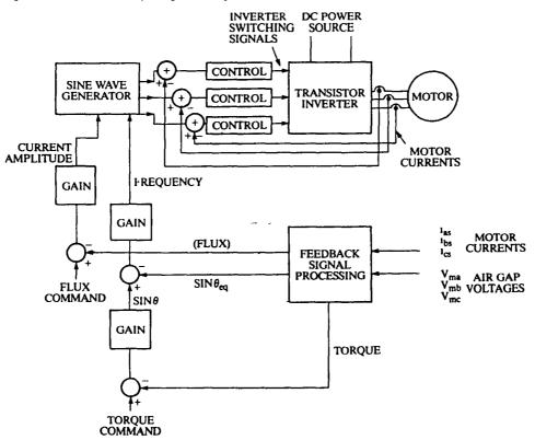
Figure 4.3.1 Overall Drive System Block Diagram
