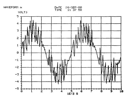
Figure 4.7-6 Motor Current in PWM Regenerative Braking Note: Current (vertical) scale factor is 80 amps/volt, time (horizontal) scale is in milliseconds.
