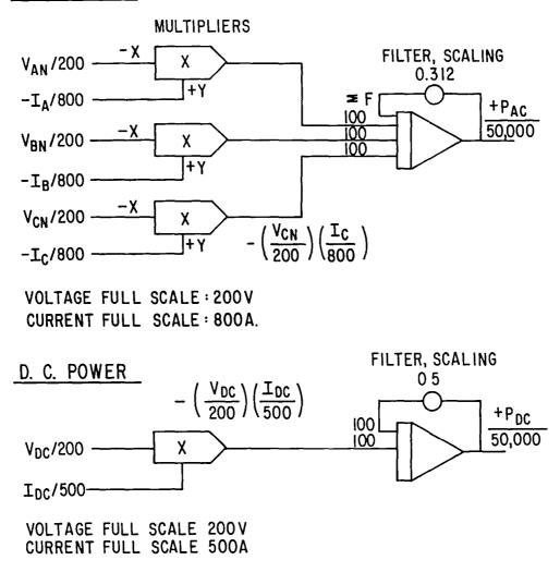
Figure 4.2-3 Analog Computer Computation Functions
