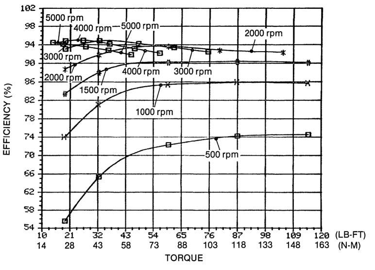
Figure 4.11-7 Controller Efficiency in Motoring Note: Speed and torque are at the gear box shaft after the 2.923:1 reduction.
