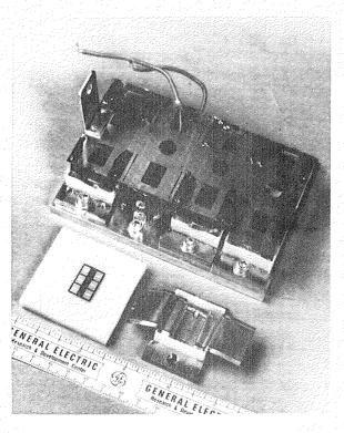
Figure 3.8.6-1 Power Module with Darlington Chip and Subscrete in the Foreground
