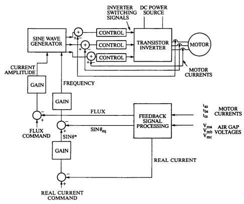
Figure 3.5.3-4 Overall Drive System Block Diagram
