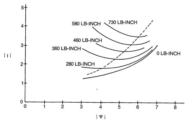
Figure 4.5-1 Motor Flux Operating Point Note: Current (vertical) scale is 80 amps/volt, Flux (horizontal) scale is in volts on the control card.
