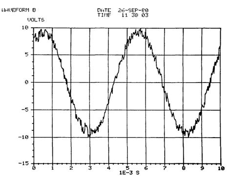
Figure 4.7-5 Motor Air Gap Flux Voltage in PWM Regenerative Braking Note: Voltage (vertical) scale is in volts, time (horizontal) scale is in milliseconds.
