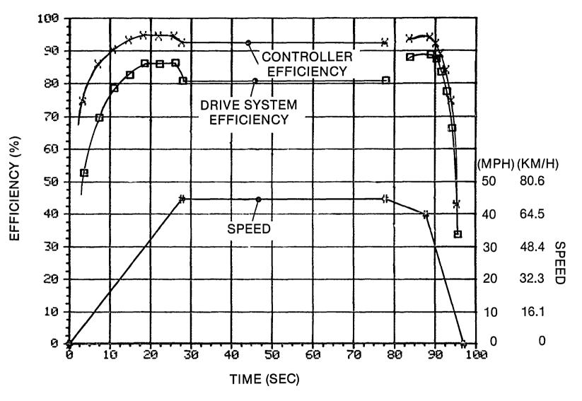
Figure 4.11-11 Efficiency over the J227 A-D Driving Cycle
