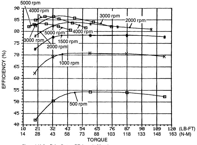
Figure 4.11-8 Drive System Efficiency in Motoring Note: Speed and torque are at the gear box shaft after the 2.923:1 reduction.
