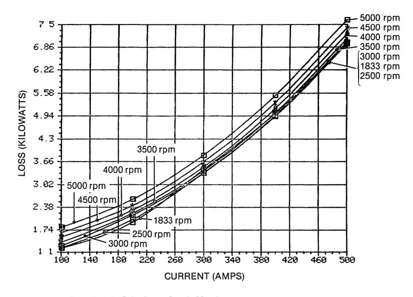
Figure 4.11-3b Drive System Loss in Motoring Note: Current is the average of the 3-phase full wave rectified motor current. Speed is at the gear box shaft after the 2.923:1 reduction.
