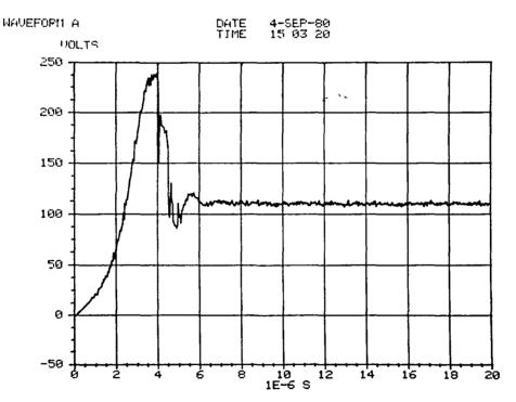
Figure 4.8-1 Power Module Voltage at Turn-off in PWM Motoring Note: Voltage (vertical) scale is in volts, time (horizontal) scale is in microseconds.
