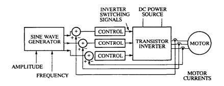
Figure 3.5.2-2 Current-Controlled PWM Block Diagram
