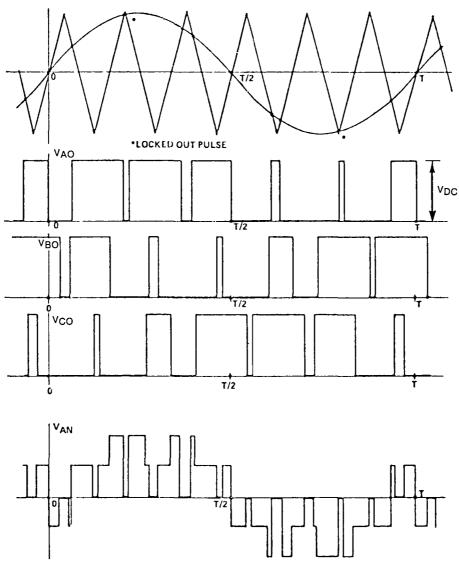
Figure 3.4.5-1 Generation of Sine Wave PWM
