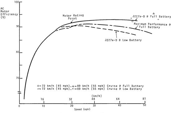
Figure 3.4.4-2 Motor Sine Wave Efficiency – Motoring
