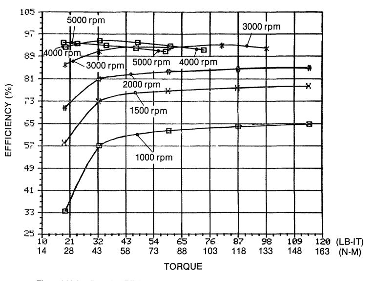
Figure 4.11-9 Controller Efficiency in Regenerative Braking Note: Speed and torque are at the gear box shaft after the 2.923:1 reduction.
