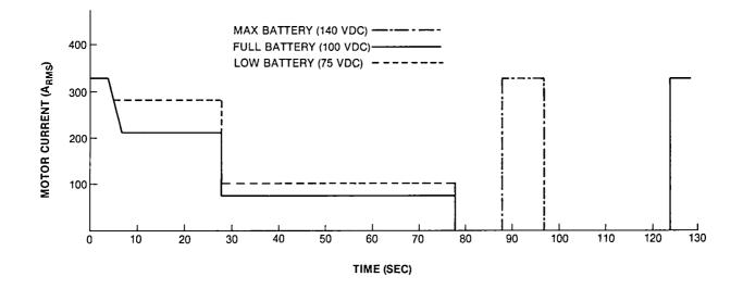
Figure 3.2.4-1 AC Motor Current for J227a-Schedule D Duty Cycle
