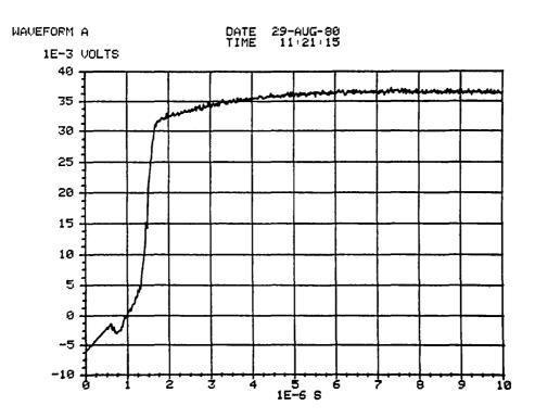
Figure 4.8-4 Power Module Base Drive Turn-on Current in Square Wave Motoring Note: Current (vertical) scale factor is 1 amp/10 millivolts, time (horizontal) scale is in microseconds.
