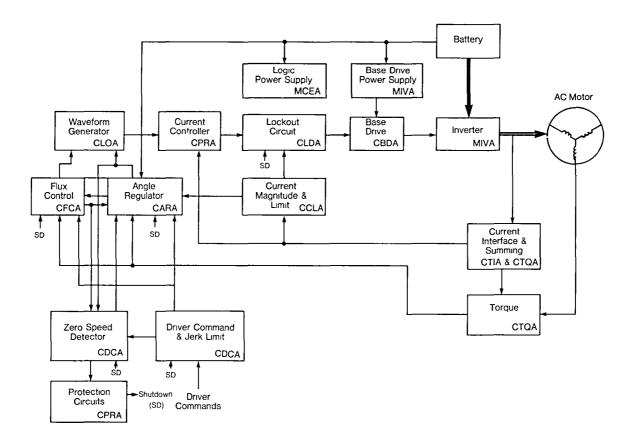
Figure 3.6-2 Control Circuit Card Block Diagram
