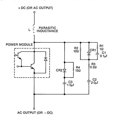
Figure 3.7.5-1 Power Darlington Transistor Snubber
