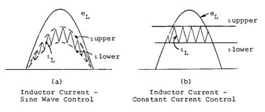
Figure 3.11.4-4 Chopper Current Controls
