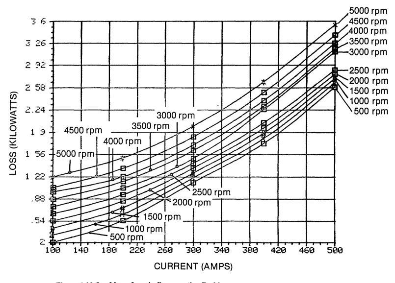
Figure 4.11-5 Motor Loss in Regenerative Braking Note: Current is the average of the 3-phase full wave rectified motor current. Speed is at the gear box shaft after the 2.923:1 reduction.
