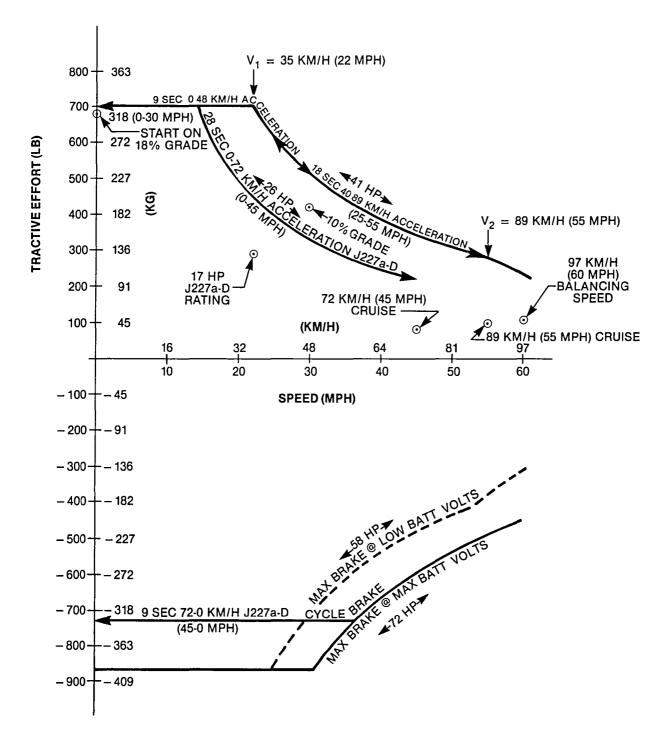
Figure 3.2.2-1 Motor Tractive Effort and Speed Requirement
