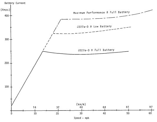
Figure 3.4.4-5 Battery Current – Motoring
