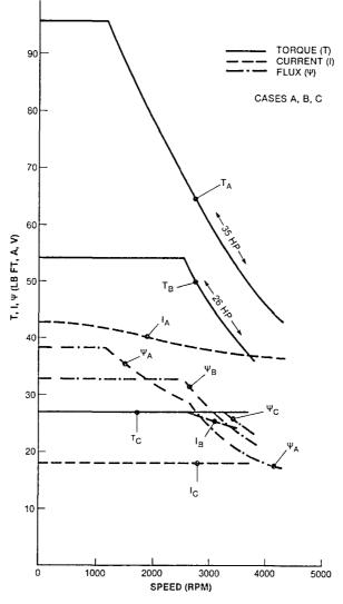
Figure 4.9-5. System Torque-Speed Performance
