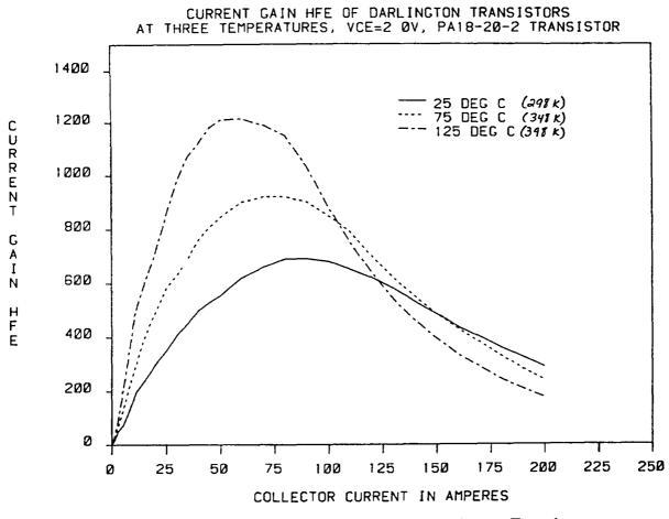
Figure 3.8.5-1 Gain Characteristic of ZJ504 Darlington Transistor
