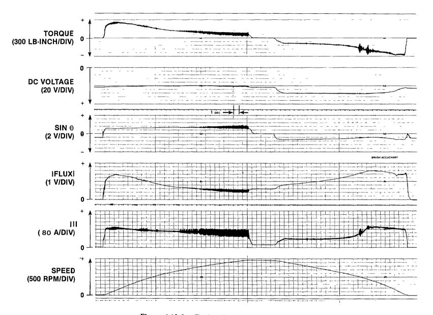
Figure 4.12-2. Typical Performance Recording with DC Voltage
