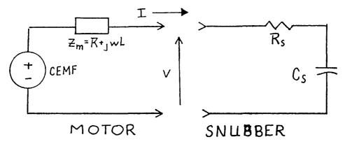
Figure 3.9.5.3-1 Snubber Equivalent Circuit
