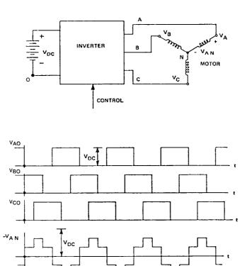
Figure 3.4.5-3 Generation of Six Step Square Wave
