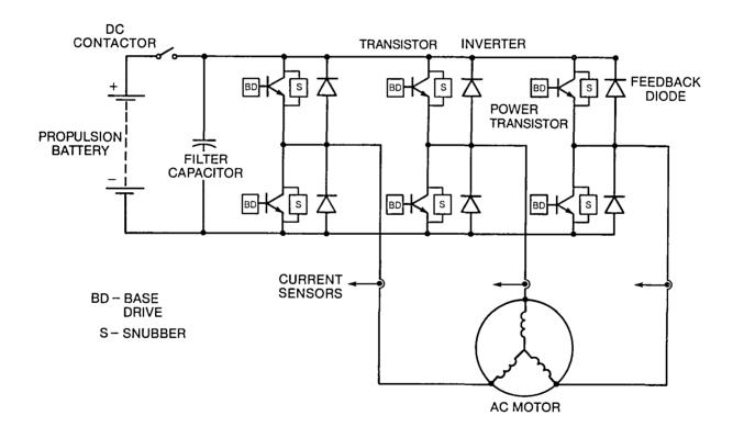
Figure 3.5.4-1 Inverter Power Circuit
