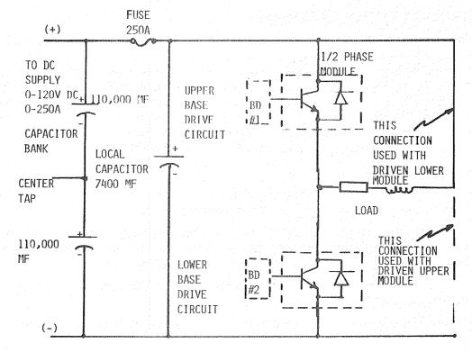
Figure 3.8.7-1 Test Circuit for Half-Phase Module
