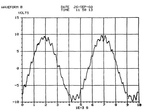
Figure 4.7-2 Motor Air Gap Flux Voltage in PWM Motoring Note: Voltage (vertical) scale is in volts, time (horizontal) scale is in milliseconds.
