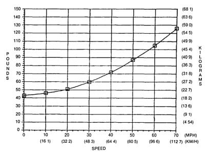
Figure A-3 Total Vehicle Friction and Windage
