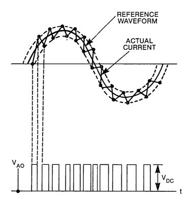
Figure 3.4.5-2 Generation of Current-Controlled PWM
