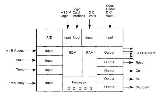
This could be implemented by a configurable controller as shown in Figure 3 9 8 8-1
