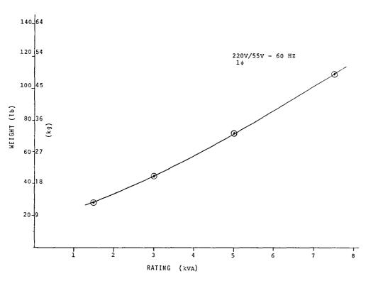
Figure 3.11.5.2-1 Transformer Weight
