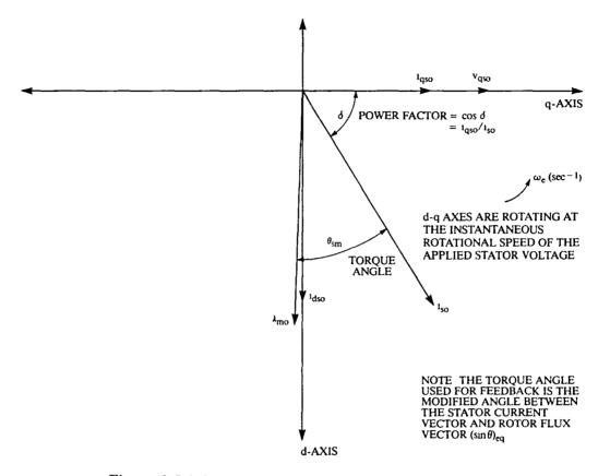
Figure 3.5.3-2 Vector Diagram of Motor Operation
