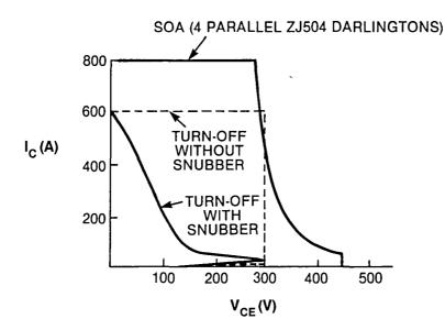
Figure 3.7.5-2 Power Darlington Transistor Turn-off Safe-Operating-Area (SOA) and Switching Locus
