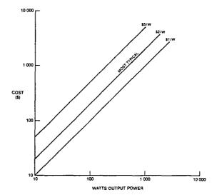
Figure E-2 Switching Power Supply Cost
