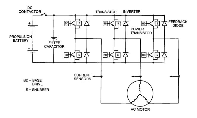
Figure 3.7-3 Inverter Power Circuit
