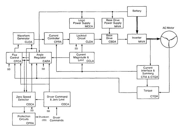
Figure 3.9.8.1-1 Simplified AC Controller Block Diagram
