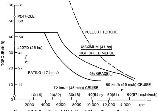
Figure 3.2.1-2 Typical High-Speed Motor Torque Requirements
