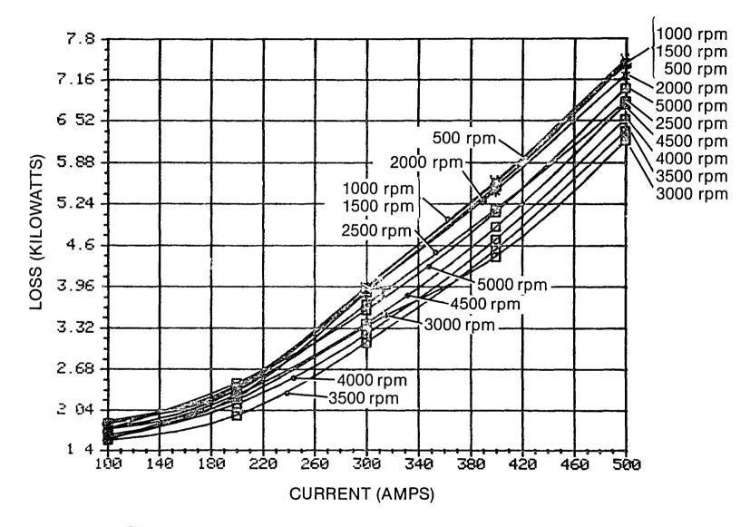
Figure 4.11-6 Drive System Loss in Regenerative Braking Note: Current is the average of the 3-phase full wave rectified motor current. Speed is at the gear box shaft after the 2.923:1 reduction.
