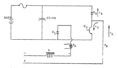
Figure 3.11.4-3 Active Components for Negative Half Cycle
