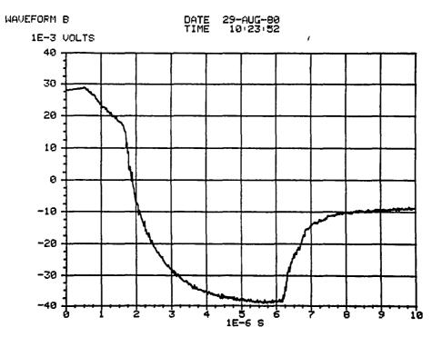
Figure 4.8-5 Power Module Base Drive Turn-off Current in Square Wave Motoring Note: Current (vertical) scale factor is 1 amp/10 millivolts, time (horizontal) scale is in microseconds.
