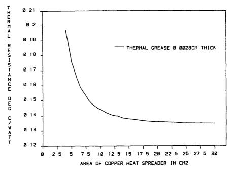
Figure 3.8.4-1 Thermal Resistance of Darlington Subscrete
