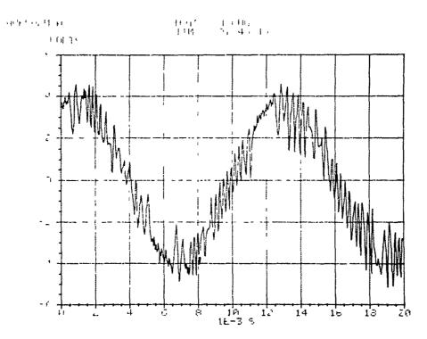
Figure 4.6-1 Motor Current in PWM Motoring Note: Current (vertical) scale factor is 80 amps/volt, time (horizontal) scale is in milliseconds.
