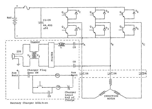
Figure 3.11.3-1 AC Controller Power Circuit with Charger
