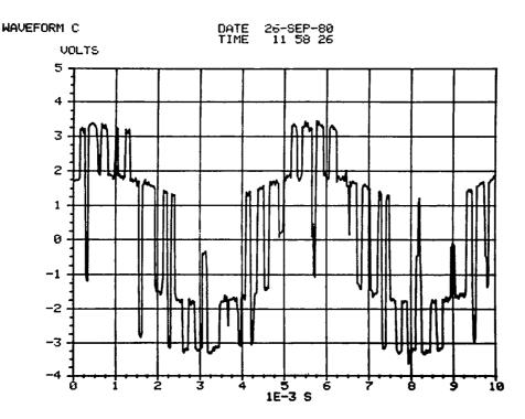
Figure 4.7-1 Motor Line-to-Neutral Voltage in PWM Motoring Note: Voltage (vertical) scale factor is 20 volts/volt, time (horizontal) scale is in milliseconds.
