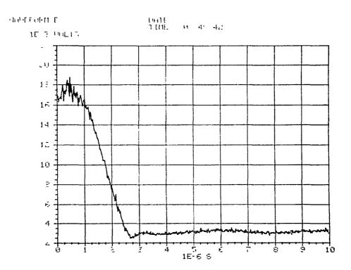
Figure 4.8-2 Power Module Current at Turn-off in PWM Motoring Note: Current (vertical) scale factor is 40 amps/millivolt, time (horizontal) scale is in microseconds. Actual zero current is at 3 millivolts in waveform.
