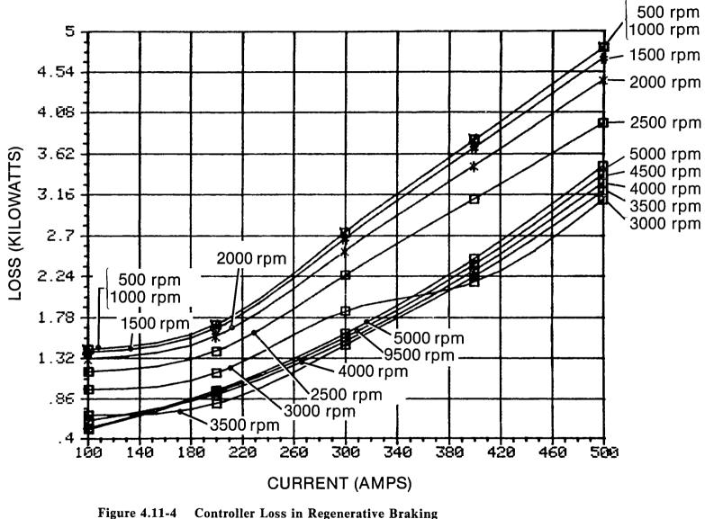
ure 4.11-4 Controller Loss in Regenerative Braking Note: Current is the average of the 3-phase full wave rectified motor current. Speed is at the gear box shaft after the 2.923:1 reduction.
