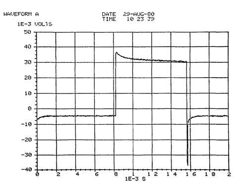
Figure 4.8-3 Power Module Base Drive Current in Square Wave Motoring Note: Current (vertical) scale factor is 1 amp/10 millivolts, time (horizontal) scale is in milliseconds.
