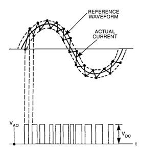
Figure 3.5.2-1 Generation of Current-Controlled PWM
