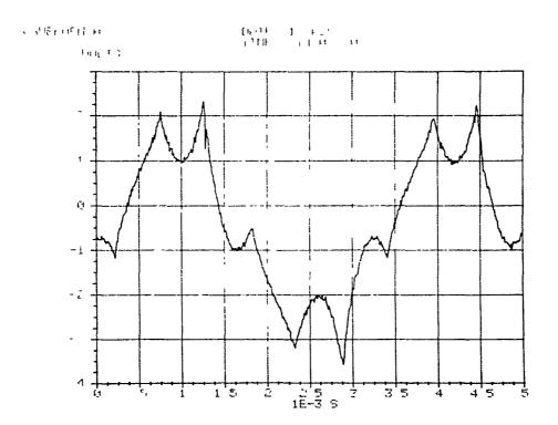
Figure 4.6-7 Motor Current in Square Wave Regenerative Braking Note: Current (vertical) scale factor is 80 amps/volt, time (horizontal) scale is in milliseconds.
