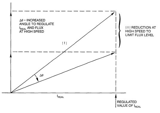
Figure 3.6.2.3-1 Regulation of Real Component of Current
