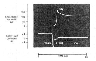
Figure 3.7.4-2 Power Darlington Turn-off with Reverse Base 2 Drive
