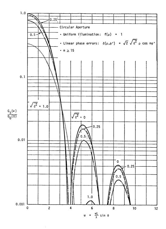
Figure 6. The effect of small-scale linear phase errors on the secondary pattern of a uniformly illuminated antenna.
