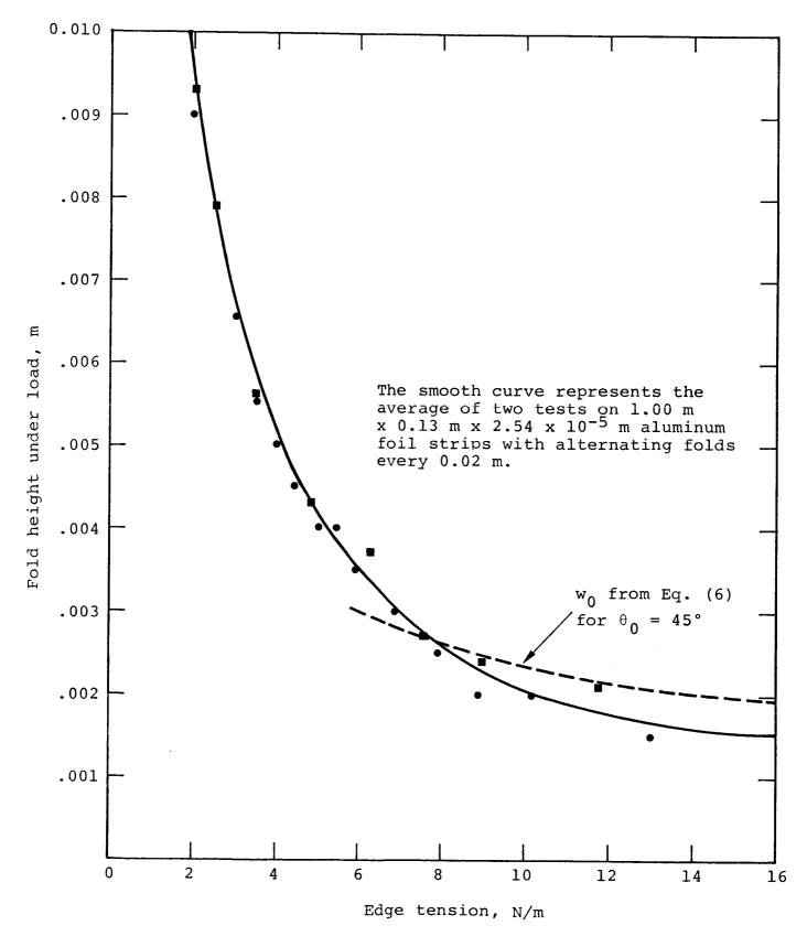
Figure 5. Fold height of folded foil under tension.
