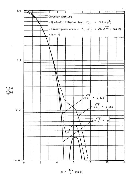
Figure 3. The effect of linear phase errors on the secondary pattern of an antenna with a quadratic illumination.
