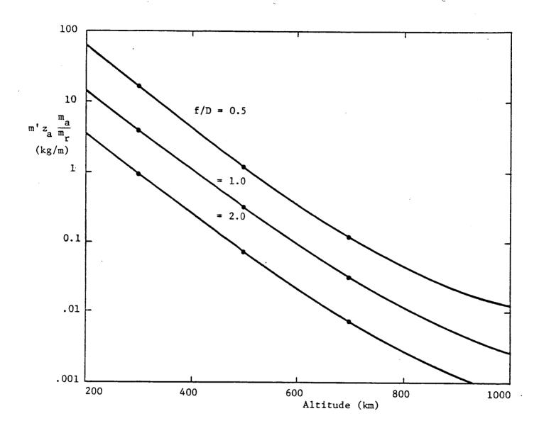
Figure 4. Minimum Value of  $m'z_a \frac{m_a}{m_r}$  required to Control Steady Pitching Moment Due to Aerodynamic Drag.
