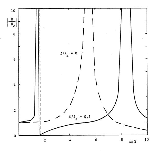
Figure E-4. Dynamic Amplification Factor for  $\alpha = 10$ .
