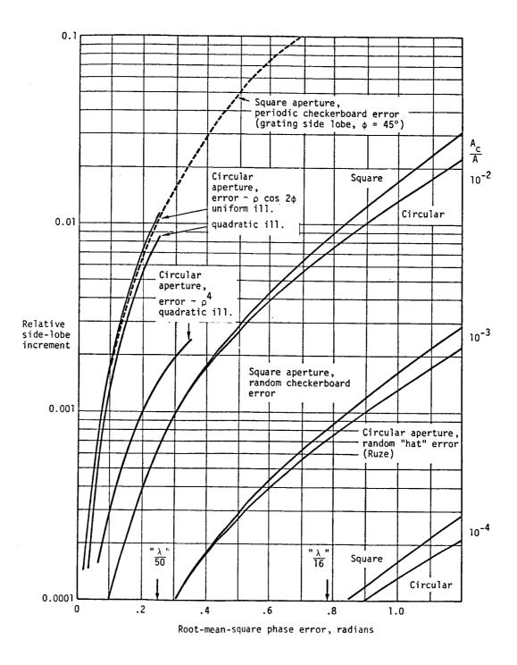
Figure 10. Effect of errors on antenna side lobes.
