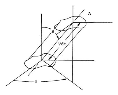
Select the lower side as the one through which the meteoroids are passing. Then all the meteoroids in the cylindrical volume shown above that have spherical-coordinate velocity components of V,  $\theta$ , and  $\phi$  pass through the area A in the unit time. Thus the total
