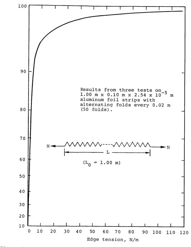
Figure 4. Extension of folded foil section under tension.
