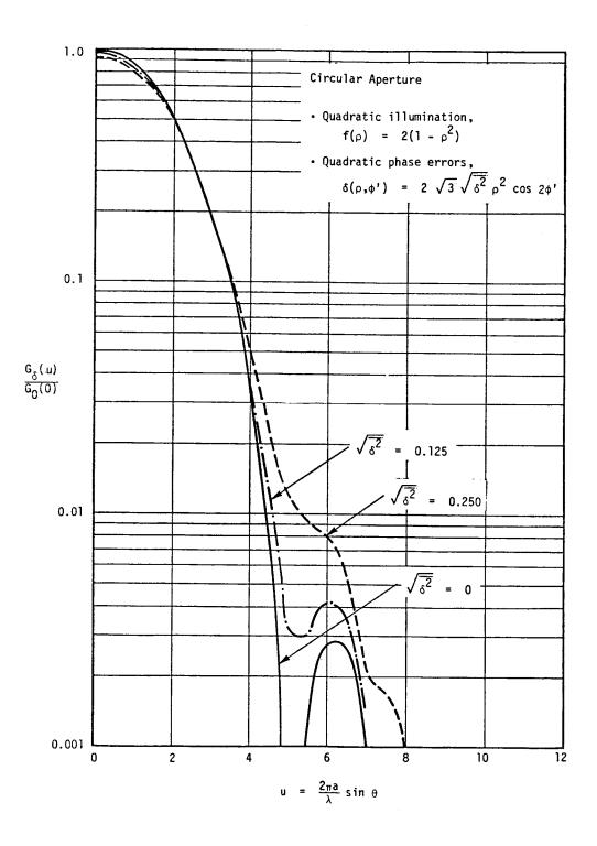
Figure 4. The effect of quadratic phase errors on the secondary pattern of an antenna with quadratic illumination.
