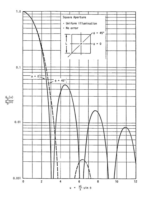
Figure 7. Secondary patterns of a square antenna array without phase errors.
