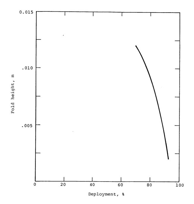
Figure 7. Deployment of a foil surface folded in two directions.
