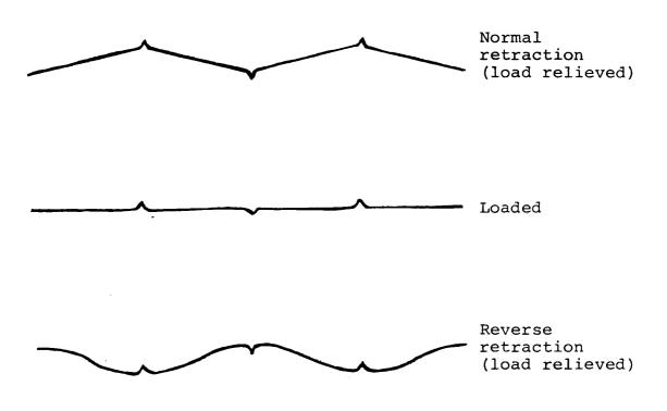
Figure A-5. Illustration of reverse retraction which occurred at high loads when load relieved (see also Figure A-4).
