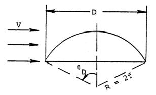
The reflector is assumed to be a segment of a sphere and to be smooth. According to Newtonian theory, the aerodynamic pressure is normal to the . surface and proportional to  $\cos^2\gamma$  where  $\gamma$  is the angle between the normal to the surface and the velocity vector. The component of pressure in the direction of the velocity vector is equal to  $\cos\gamma$  times the normal pressure. Thus, the total drag force
