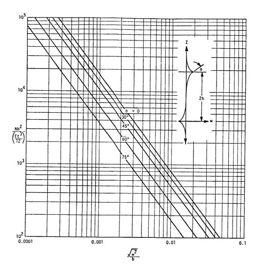
Figure 2. Membrane tension required to flatten creased film.
