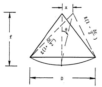
A simple geometrical analysis shows that, for  $\varepsilon \ll 1$ , the error in pointing accuracy due to differential thermal strain is
