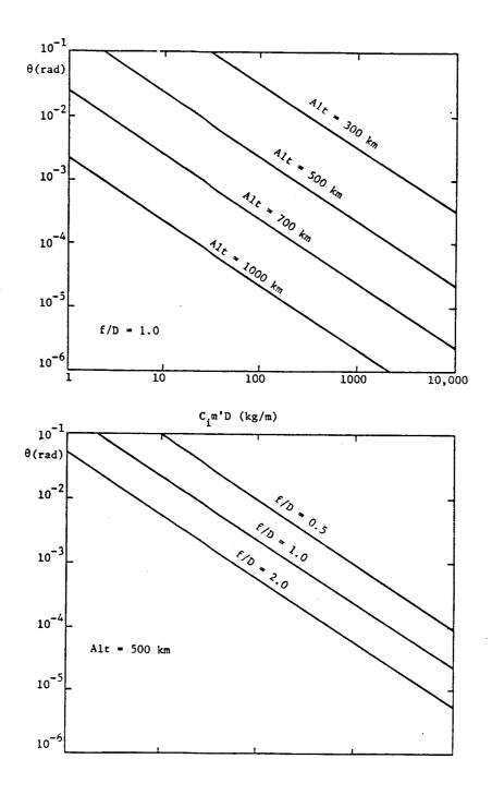
Figure 3. Steady Pitch Angle Due to Aerodynamic Drag with Gravity Gradient Stabilization.
