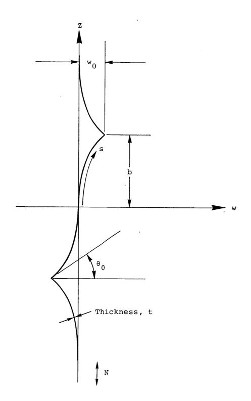
Figure 1. Alternating parallel creases in a film or foil.
