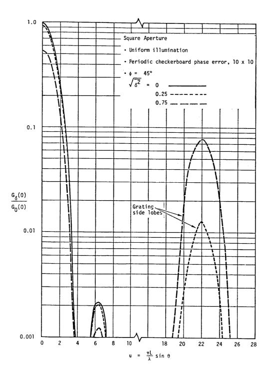
Figure 8. Secondary patterns of a square antenna array with checkerboard phase errors.
