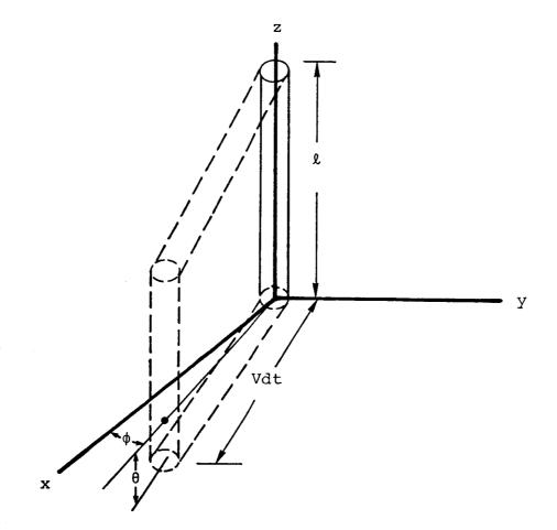
In the same way as before, all the meteoroids with velocitycomponent coordinates of V,  $\theta$ ,  $\phi$  in the above volume of VLd sin  $\theta$ will hit the cylinder in a unit time. All meteoroids with velocitycomponent coordinates of V,  $\theta$ ,  $\phi$  outside of that volume will miss the cylinder. Thus, the total rate of hits from all directions is
