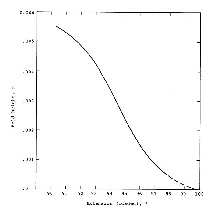
Figure A-12. Fold height vs. percent extension (loaded) (from data of third test).
