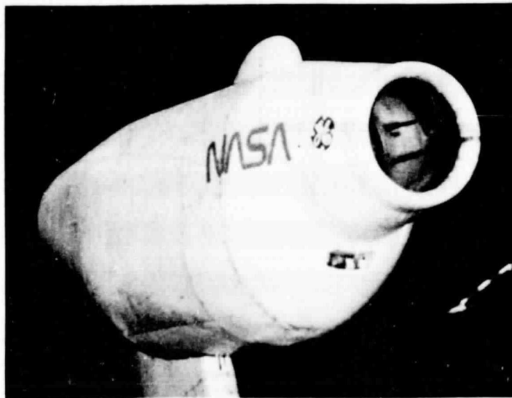
Figure 17. Photograph of JT15D/STOL Hybrid Inlet with Flight Lip and Fairings.
