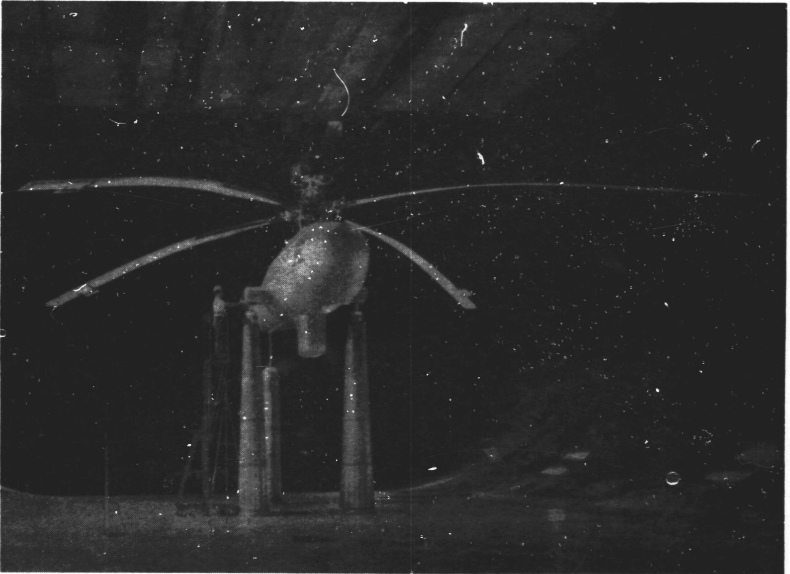
Figure 1. MCTR in 40 x 80-foot Wind Tunnel.
