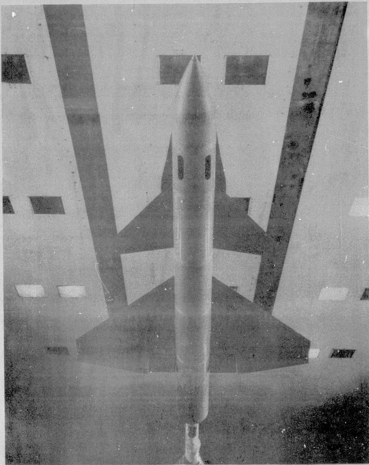
Figure 2.- Original close-coupled wing-canard configuration from reference 4, installed in V/STOL tunnel.
