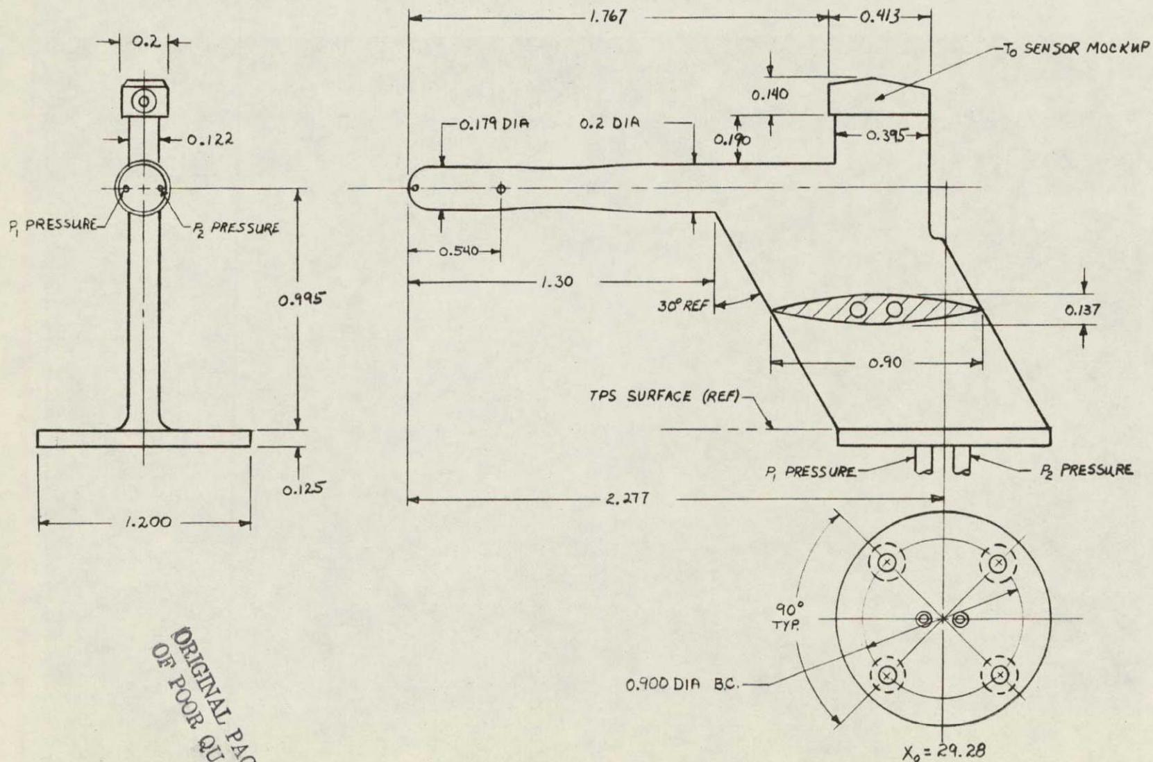
c. Air Data System (ADS) Probe Detail (0.2 Scale)
