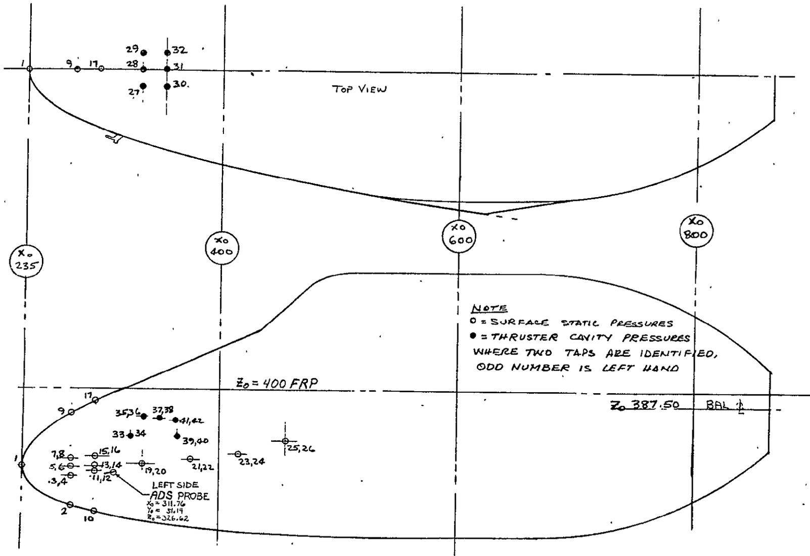
a. Thruster Cavity, Surface Static Pressure Tap and ADS Probe Locations
