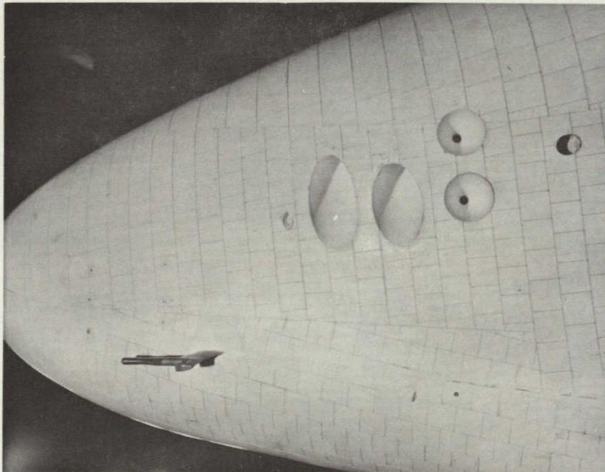
d. Left ADS Probe Pitot/Static Sensor
