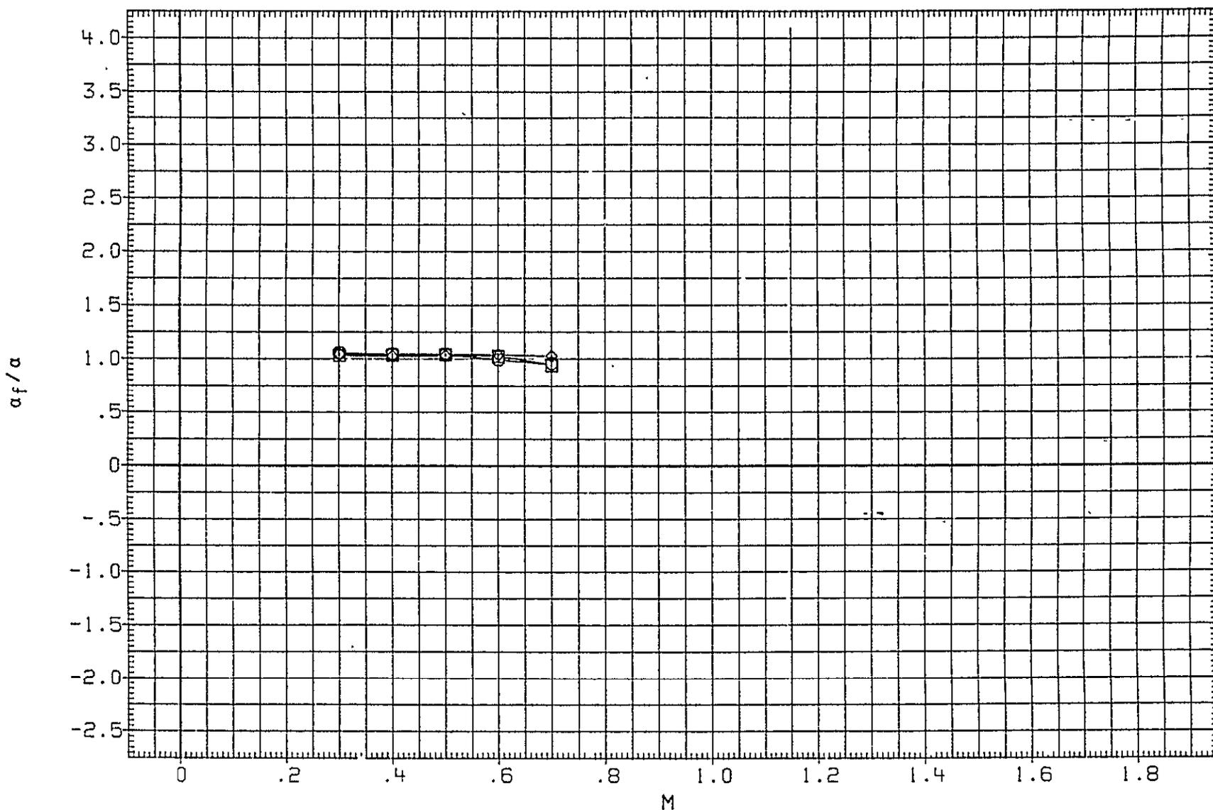
FIG. 10 MACH NUMBER EFFECT ON RATIOS OF MEASURED TO ACTUAL ANGLES OF ORBITER
