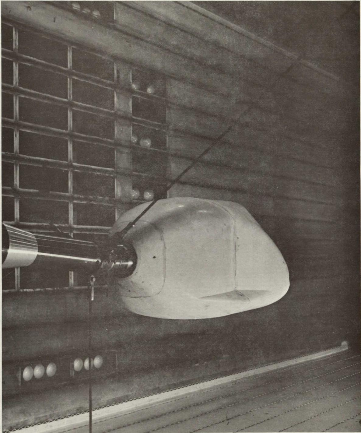
b. Three-Quarter Rear View of Model 57-0 in the ARC 14 foot Wind Tunnel
