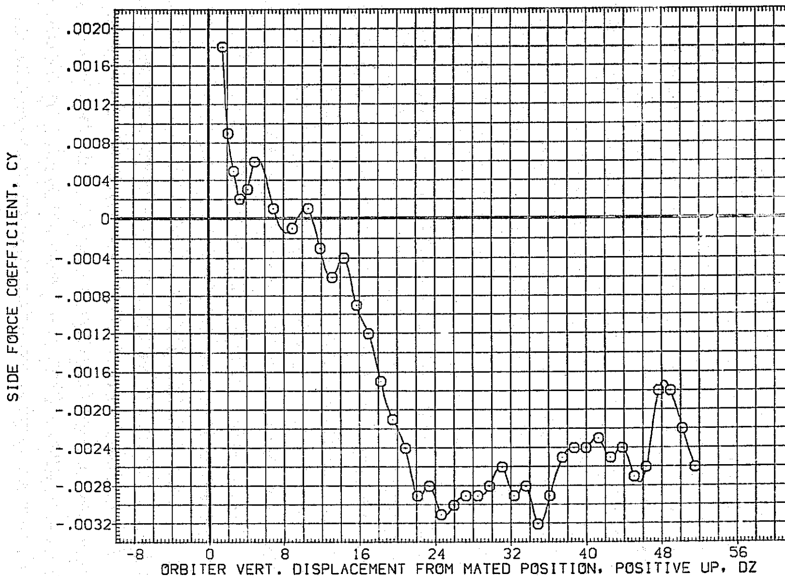
FIG.179 CARRIER DATA, ORB. PROXIMITY, ALPHAC=2, IORB=6, BETAC=0, BETA0=0, RFE075
