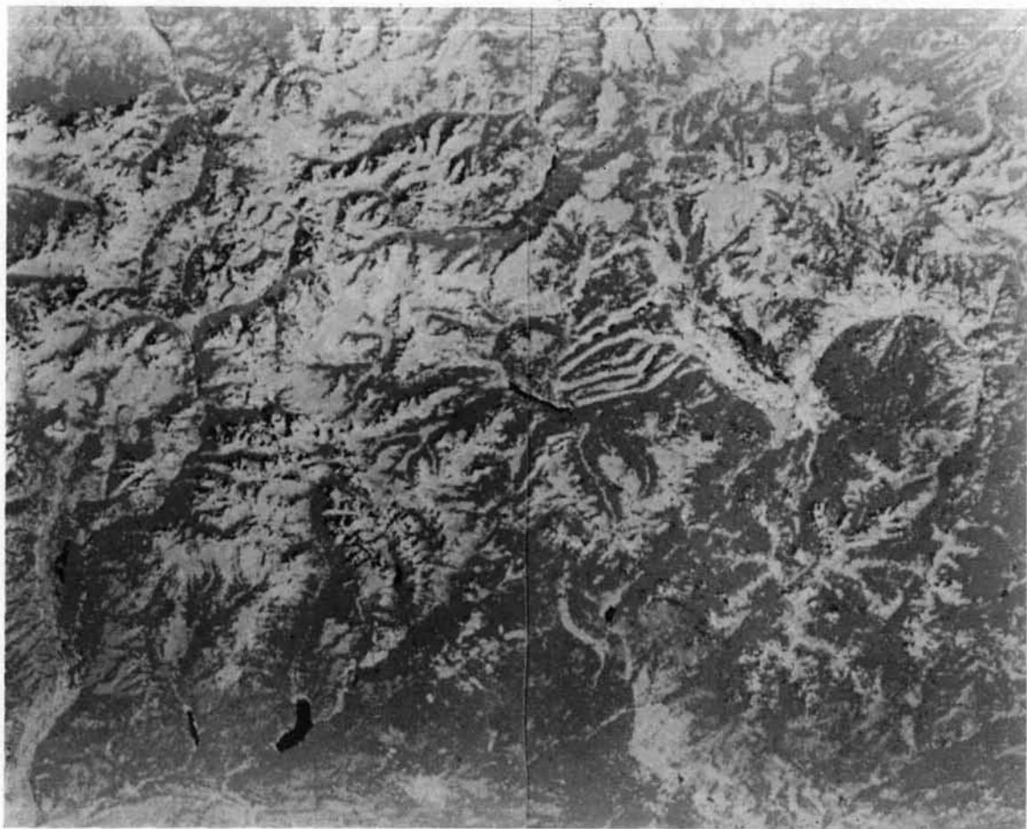
Figure A.17. Image from the digital display of the San Juan Mountain test site computer classification of level I. Black is water and terrain shadow, dark gray is coniferous forest, medium gray is deciduous forest, light gray is grass and cropland and white is barren.
