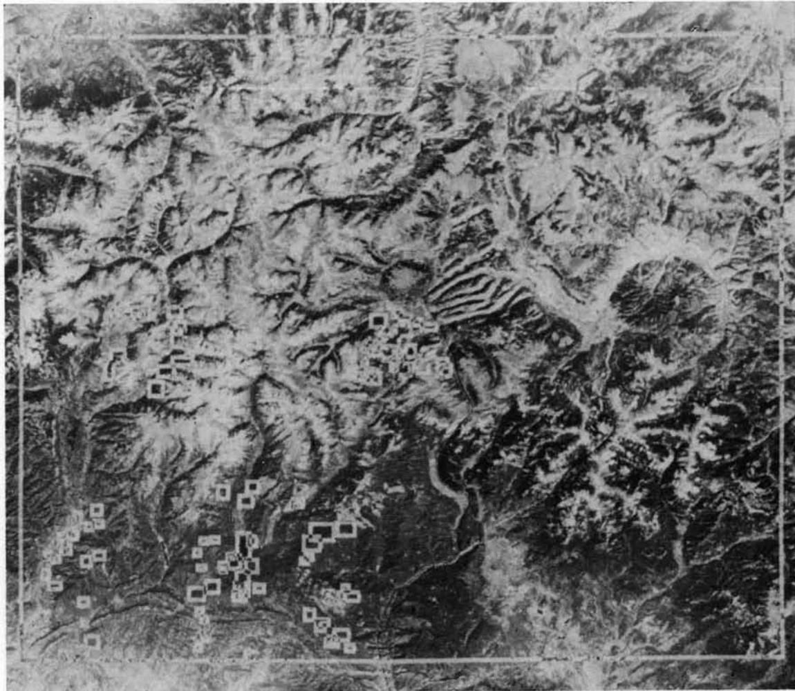
Figure A.18. ERTS-1 MSS Band 5 (0.60-0.70um) grayscale image (frame 1425-17190) of the San Juan Mountain test site showing the location of the test fields used to evaluate the classification accuracy.
