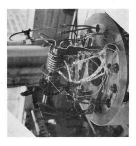
Heat Pipe 14 Mounted on Test System
