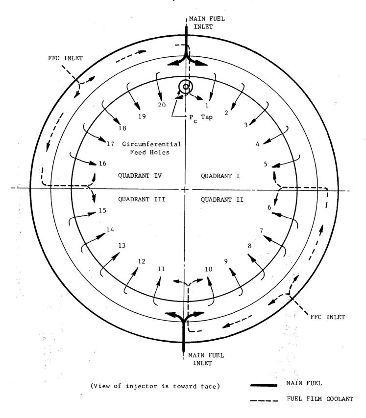
Schematic Diagram of Fuel Distribution Circuits
