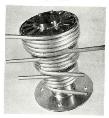
Figure 15 - Heat Pipe 8 After Assembly
