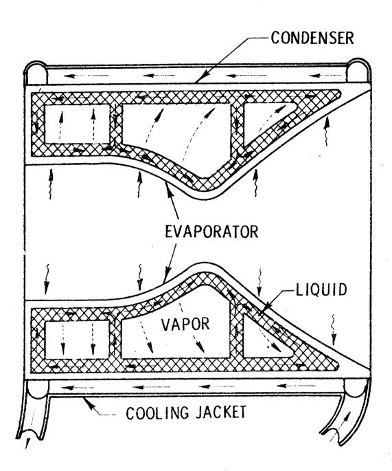
Regeneratively Cooled Heat Pipe Thrust Chamber Concept
