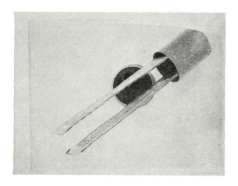
Figure 18 - Heat Pipe 9A Feeders and Condenser Wick
