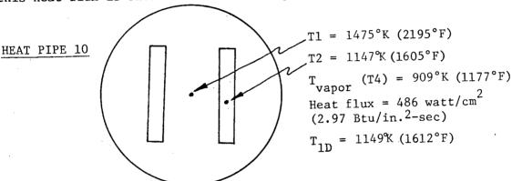
The high evaporator midpoint temperature between feeders did not develop suddenly as a result of a temperature excursion but was consistently higher than expected as the heat flux was increased. This is shown by the test data graph of Figure 28 which shows measured and predicted values as a function of heat flux. The wall temperature beneath the feeder appears normal throughout the test.
