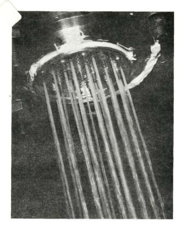
OXIDIZER CIRCUIT COLD FLOW SETUP Fluid: Water
