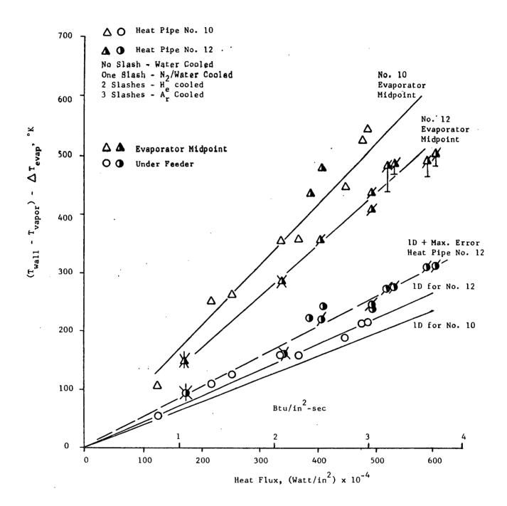
Comparison of Heat Pipe No. 12 and Heat Pipe No. 10 Test Data 148
