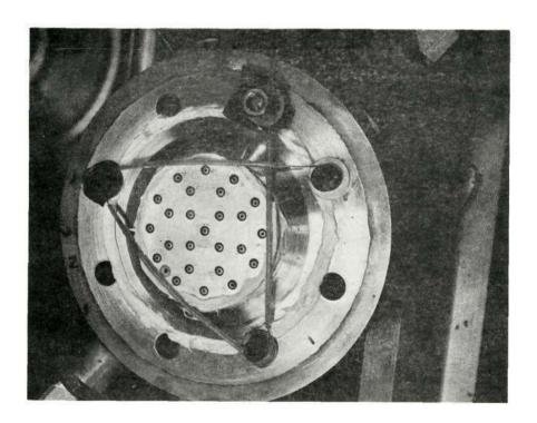
FUEL CIRCUIT COLD FLOW SETUP (Dummy Face Plate)
