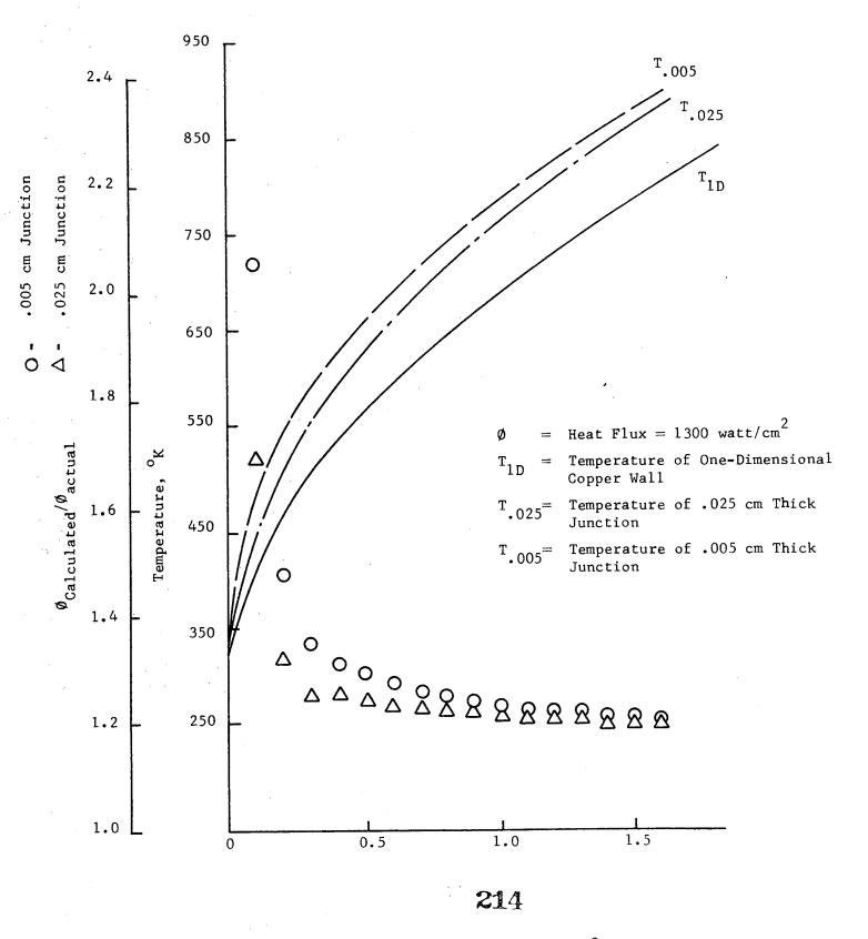
Figure B3 - Error Analysis for 1300 watt/cm<sup>2</sup> Heat Flux
