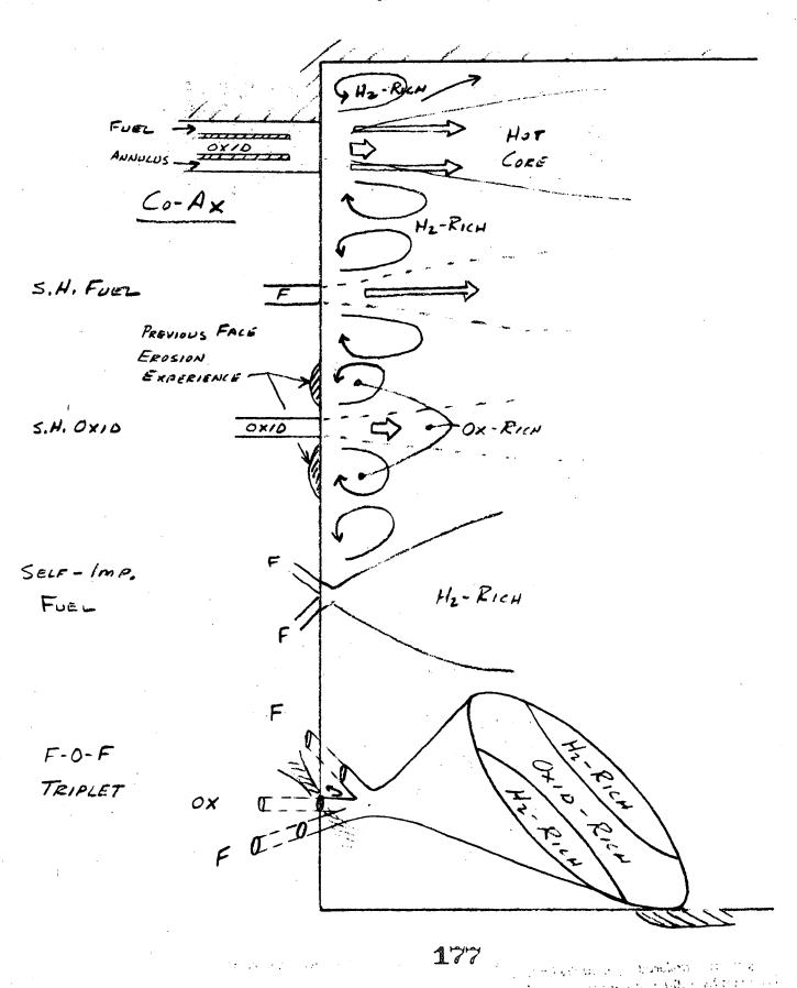
Injection Element/Face Compatibility Characteristics
