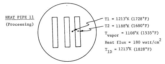
The unit was then oriented to a horizontal position and operated to 478 watt/cm<sup>2</sup> (2.93 Btu/in.<sup>2</sup>-sec) heat flux. The test was terminated at this point because the evaporator wall temperature was becoming excessive and sufficient data had been obtained to evaluate the heat pipe performance. The test data at the maximum heat flux condition are summarized in the following sketch, and the evaporator wall temperatures are shown as a function of heat flux in Figure 32.
