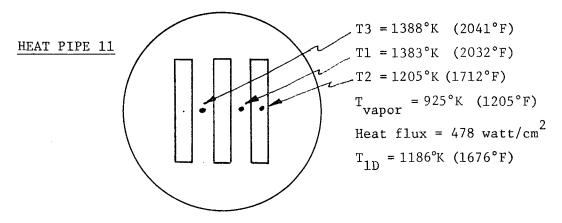
The wall temperature data show that at the maximum heat flux the evaporator wall was much hotter at the midpoints between feeders than directly under the feeders. One of the midpoint temperatures, T1, showed nearly normal behavior up to  $350 \text{ watt/cm}^2$  heat flux but the other, T3, was consistently high. The wall temperature under the feeder appears normal. Therefore, these
