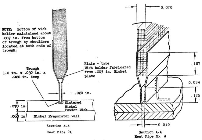
Heat Pipe 9 and 9A Evaporator/Feeder Joint Detail
