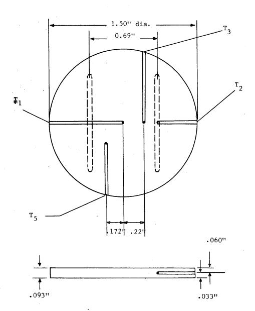
Thermocouple Locations, Heat Pipe No. 12
