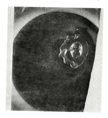
Figure 16 - Heat Pipe 8 Evaporator Wall Burnout
