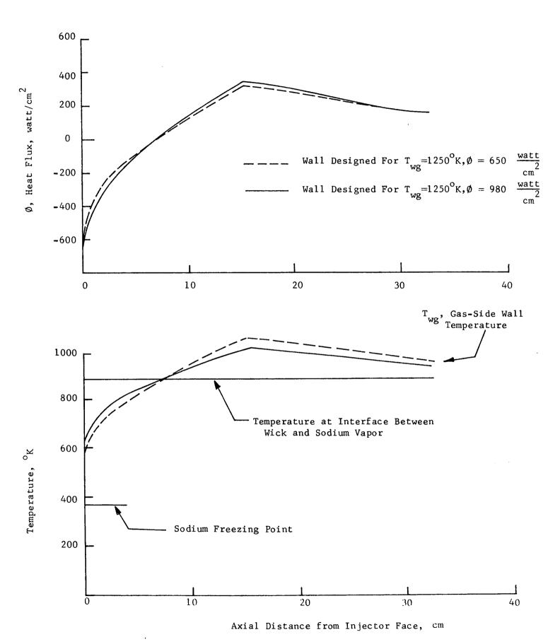
Wall Temperature and Heat Flux Distribution Figure 79
