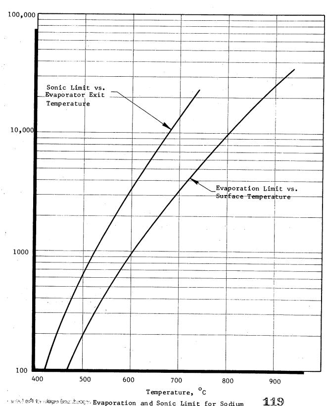
Heat Flux, watts/cm<sup>2</sup>
