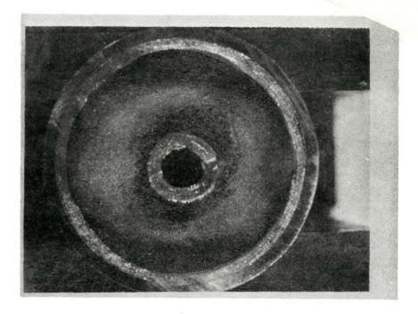
Figure 17 - Heat Pipe 8 Evaporator (Post Test)
