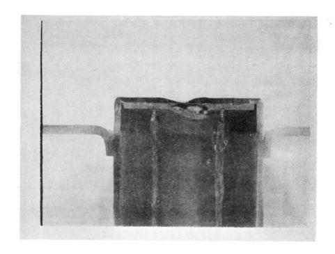
Figure 21 - Cross Section of Burnout Area, Heat Pipe 9A
