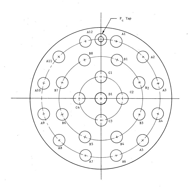
Orifice Nomenclature,  $FLOX/H_2$  Injector
