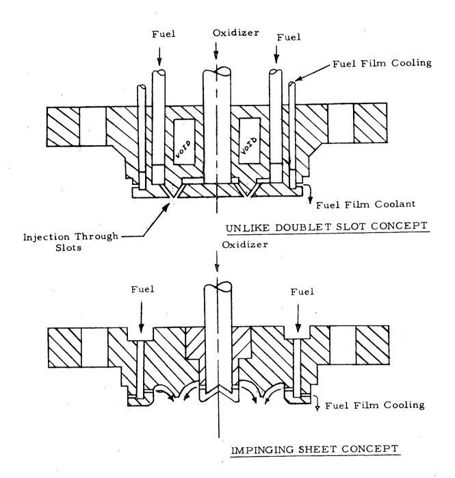
Impinging Sheet and Unlike Doublet Slot Injector Concepts
