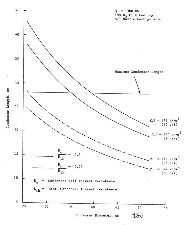
Initial Thermal Design Results for the Cooling Jacket
