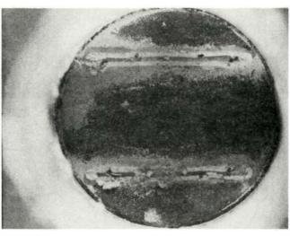
EVAPORATOR (Liquid Return Feeders Removed) Figure 41. Posttest Photographs of Heat Pipe 12 Components
