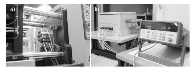
Figure 2. a) Slit die fixed to the mounting plate of the injection molding machine and b) data acquisition equipment
