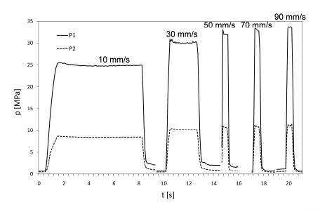
Figure 3. Recorded pressure curves with slit h = 1 mm for PP-2 at 200 °C and injection rates 10, 30, 50, 70 and 90 mm/s. The curves are from separate tests but plotted together to demonstrate the time scale at various injection rates
