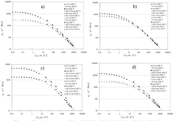
Figure 4. Viscosity curves at 200 and 230 °C a) PP-1, b) PP-2, c) PS-1, d) PS-2
