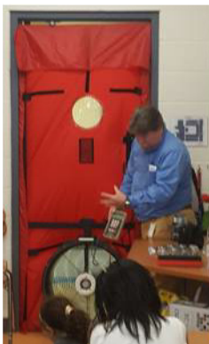
NJ Natural Gas auditor displaying a blower door.
