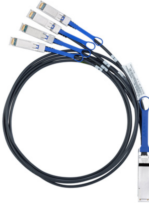
Figure 20: Breakout or Fanout Cable
