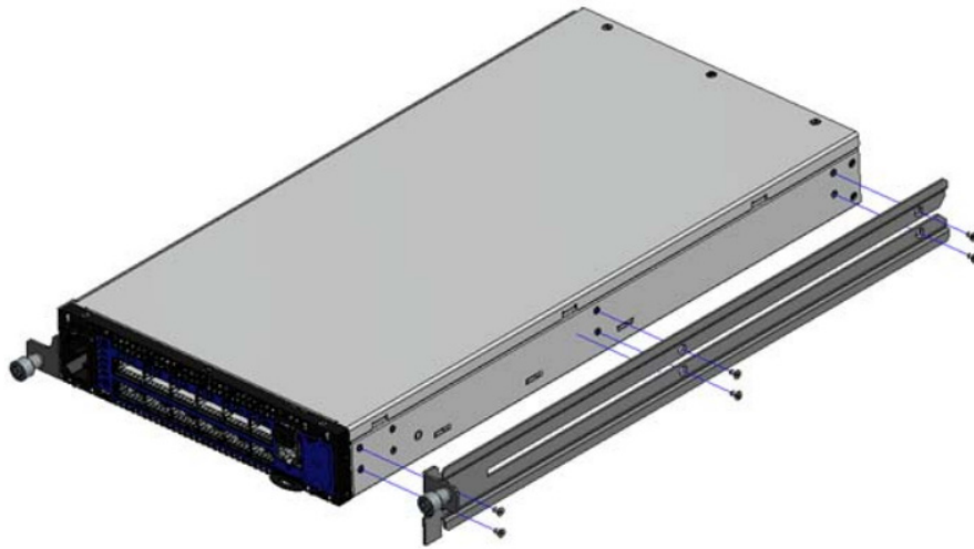
Figure 12: Screw on the System Mounted Rails
