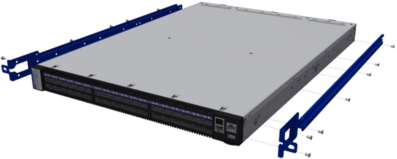
Figure 5: Screwing on the Rail
