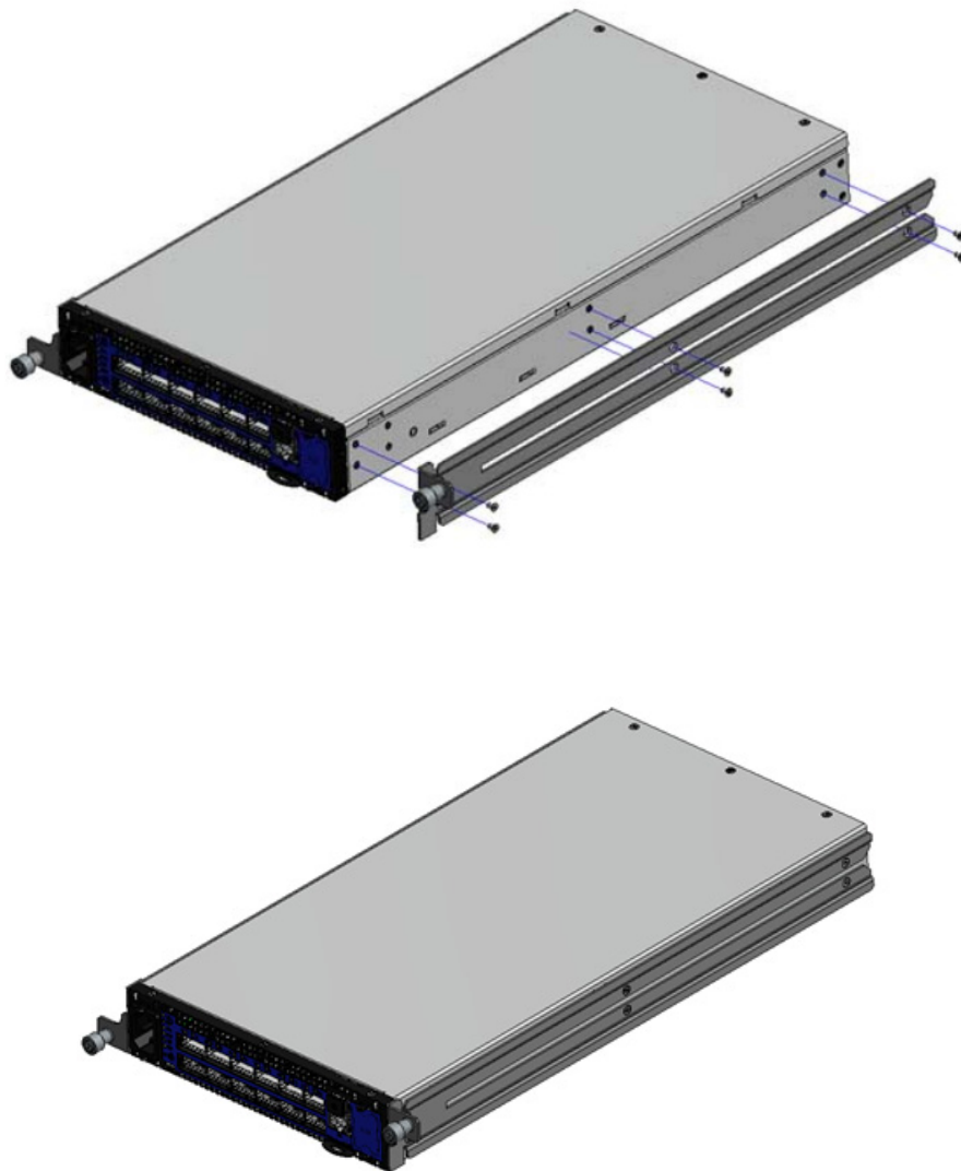
Figure 12: Screw on the System Mounted Rails
