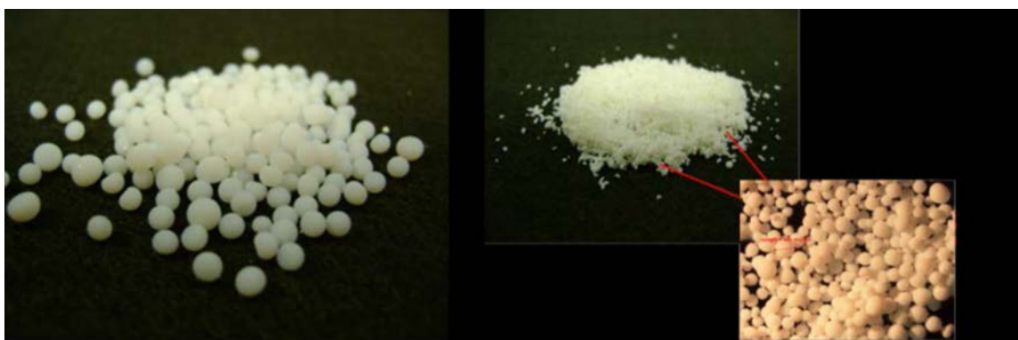
Figure 2: AFA sorbent in bead form
