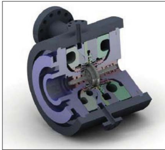
Figure 1: Cross-sectional model of a single-stage supersonic compressor
