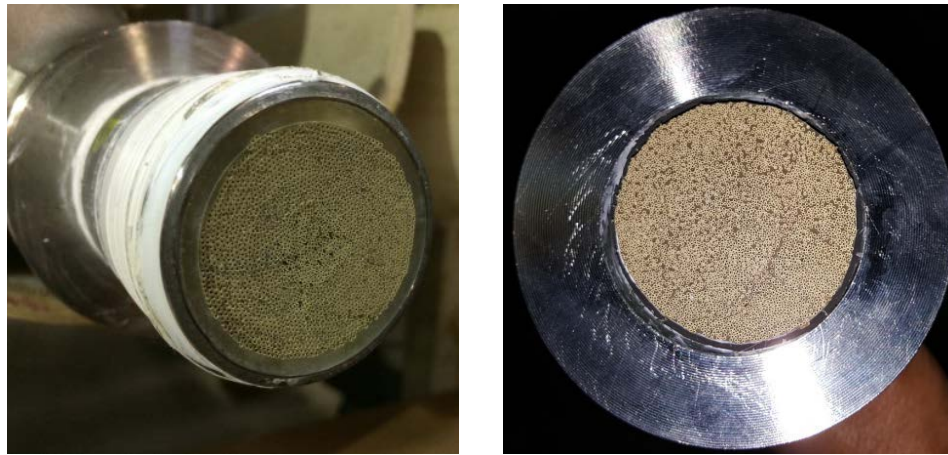
Figure 3: Photographs of PBI asymmetric hollow-fiber modules, actual 2" module (left) and 4" potted module cross-section (right)
