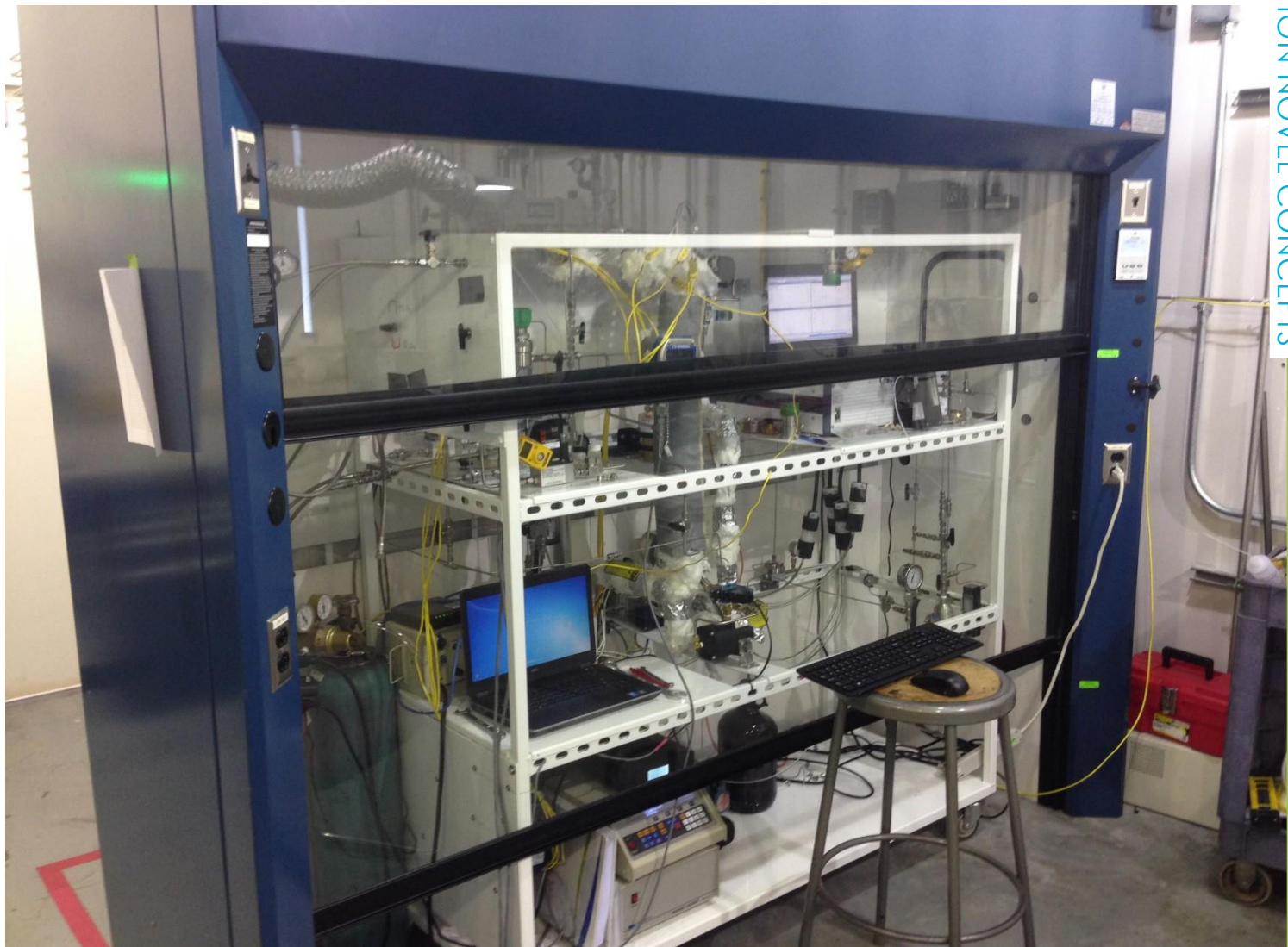
Figure 2: SR's bench-scale CO 2 capture skid
