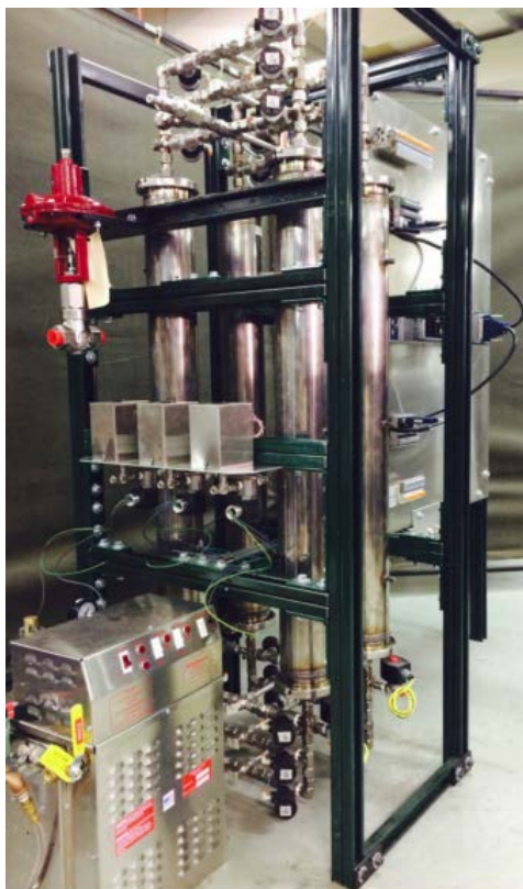
Figure 3: 4-bed VSA prototype
