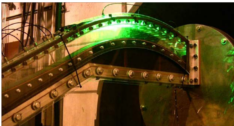
Figure 2: Bench-scale ICES test apparatus illuminated with laser sheet
