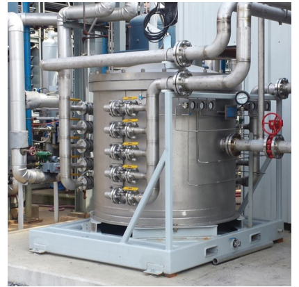
MTR's Polaris plate-and-frame membrane module
