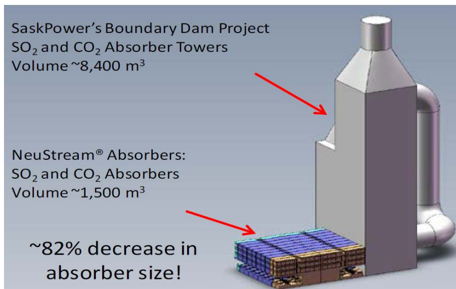
Figure 5: CO 2 Absorber size comparison: 110-MW (net) NeuStream® vs. CanSolv's 110-MW (net) SaskPower Boundary Dam Unit #3 project (includes flue gas desulfurization, CO 2 and amine wash absorbers)
