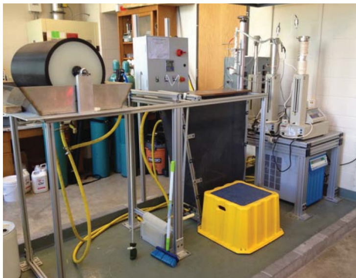
Figure 2: Georgia Tech Hollow Fiber Fabrication Line
