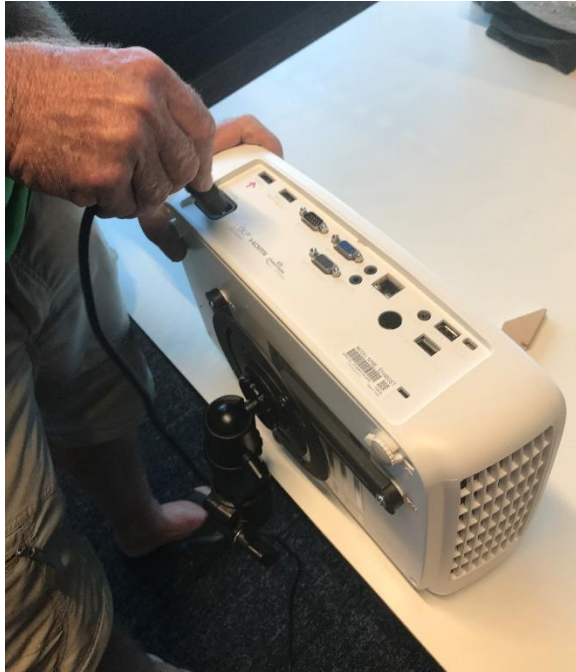
Figure 55. Plug power cord into projector socket.
