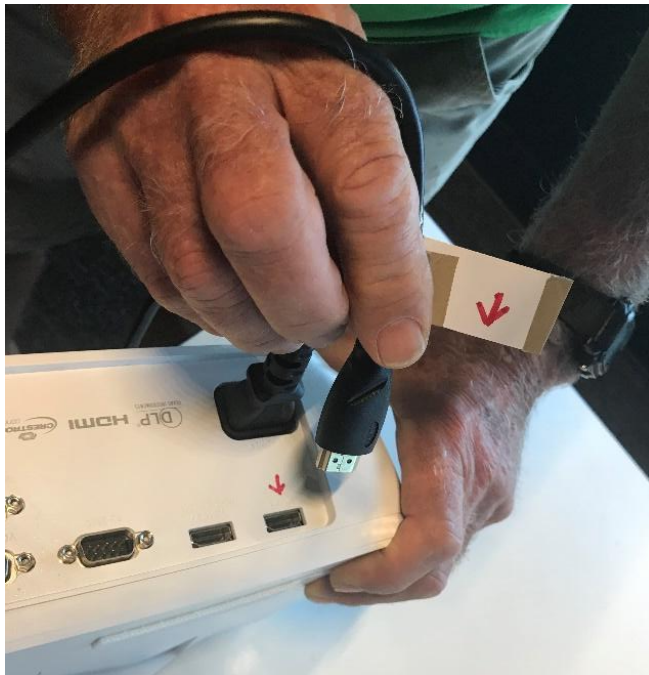
Figure 56. Plug HDMI lead into socket on far left at back, marked with a red arrow.
