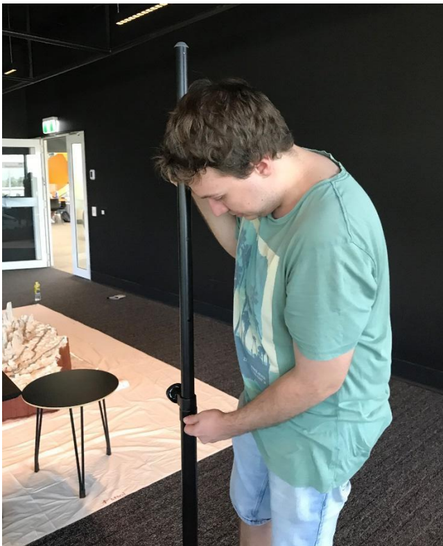
Figure 39. Raise the inner section to its full height and lock into place with small knob.
