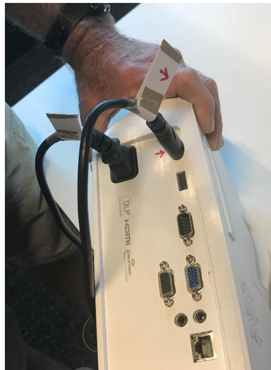
Figure 56. Plug HDMI lead into socket on far left at back, marked with a red arrow.
