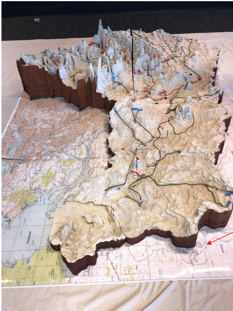
Figure 28. Western and eastern halves of the 3D map joined, showing misalignment with the underlying paper map.
