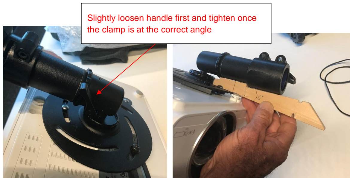
Figure 54. Adjust clamp to correct angle using the wooden tool.
