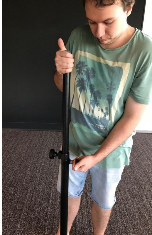
Figure 38. (a) Undo the lock (large knob) and then (b) pull out the smaller knob while raising the inside section.
