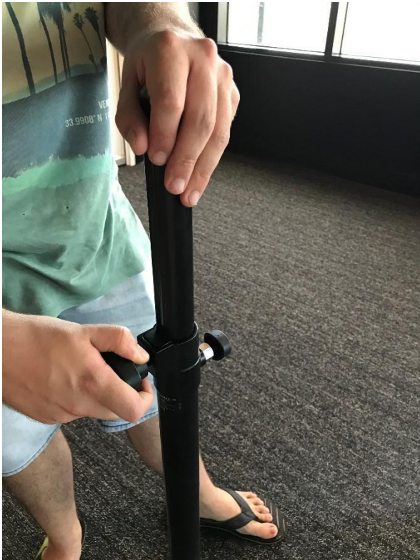
Figure 38. (a) Undo the lock (large knob) and then (b) pull out the smaller knob while raising the inside section.
