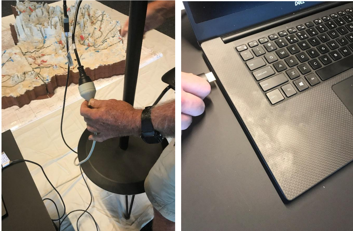
Figure 63. Plug in the power cord to the long lead and the HDMI lead to the computer.
