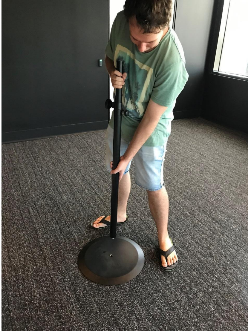
Figure 37. Screw the projector stand pole into the base.
