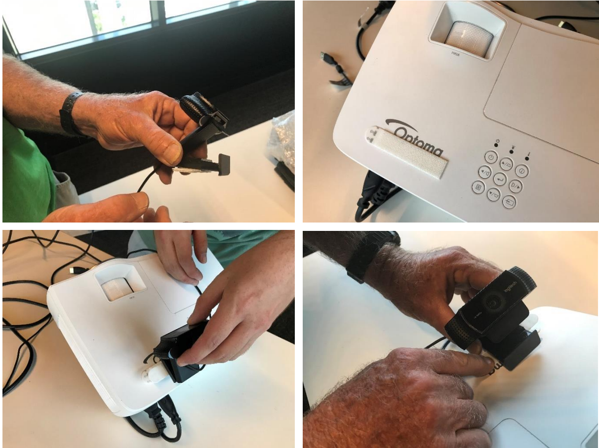
Figure 57. Attach camera by the special velcro tape and press down firmly on both sides and middle.
