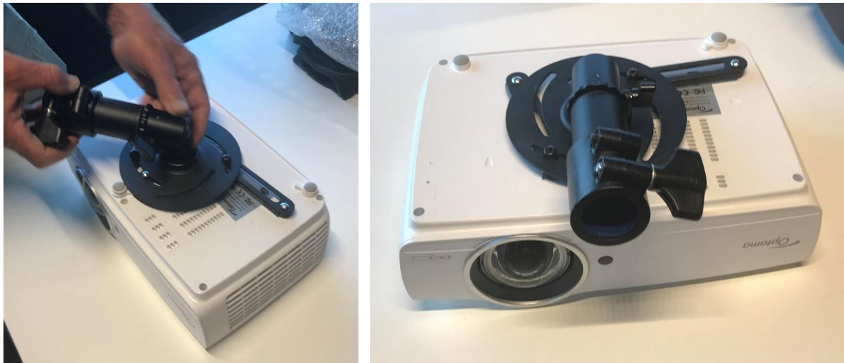
Figure 53. Attach clamp to mount on the top of the projector.
