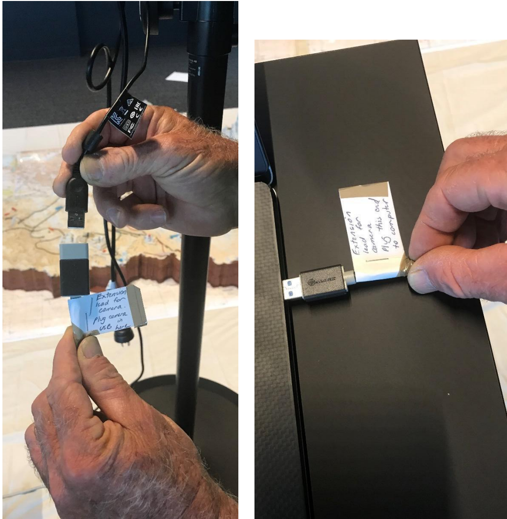
Figure 62. Plug camera lead into the USB extension, and the USB extension into the computer.
