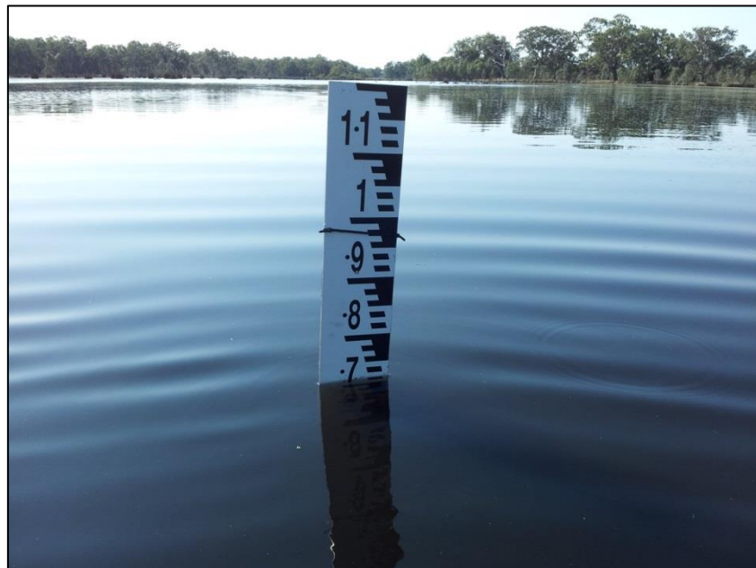
Figure 21 – The gauge board in September 2013, showing the increments used for measuring water depth
