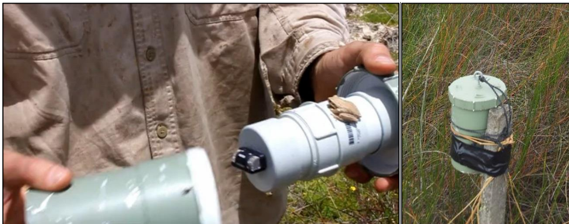
Figure 22 – A frog audio recording device is contained within this weatherproof housing
