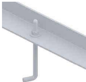
core drill and mix concrete to anchor J-Bolts
