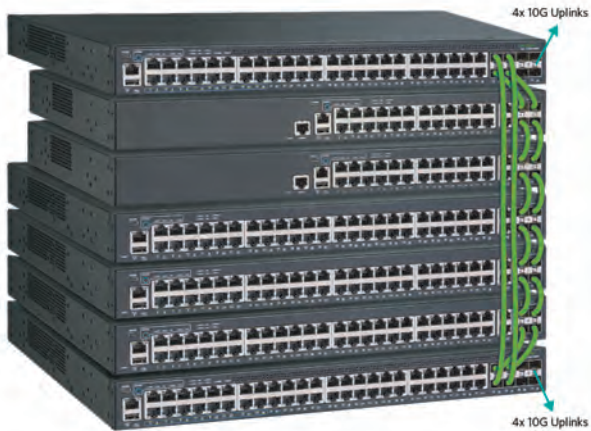
Figure 1: Up to 12 Access Networks ANX 7150 Switches can be stacked together using up to four SFP+ 10 Gbps ports per switch for a fully redundant backplane delivering 480 Gbps of aggregated stacking bandwidth.
