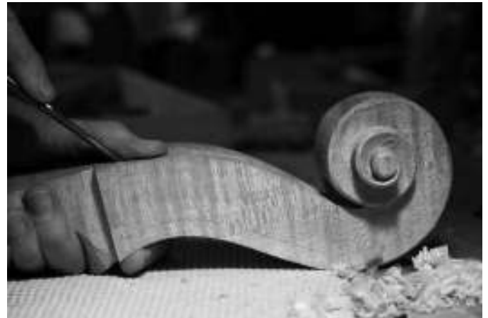
Samuel Zygmuntowicz carving a cello scroll: a design based on old geometrical proportions, with a practical purpose. Photo credit: Lilian Finckel, 2016
