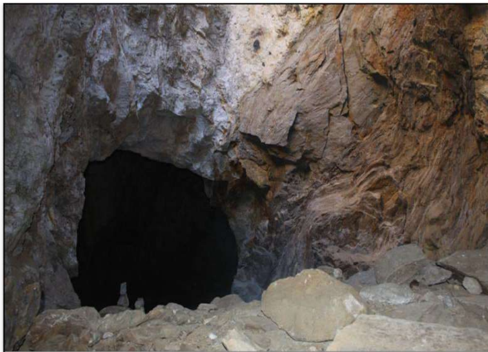
Figure 3.6 Glory hole with pegmatite footwall contact above opening
