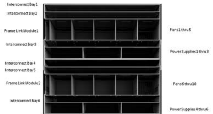
HPE Synergy 12000 Frame - Rear View
