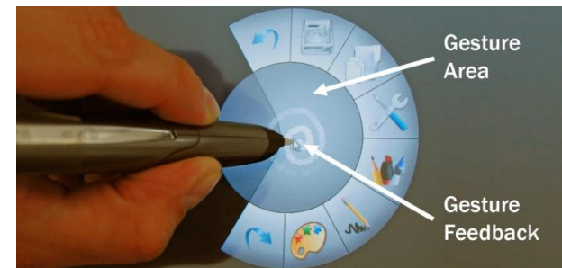
figure 6: Users can perform gestures on the circular gesture area inside the menu.
