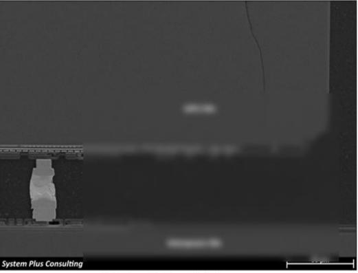
GPU Cross-Section - SEM View ©2021 by System Plus Consulting
