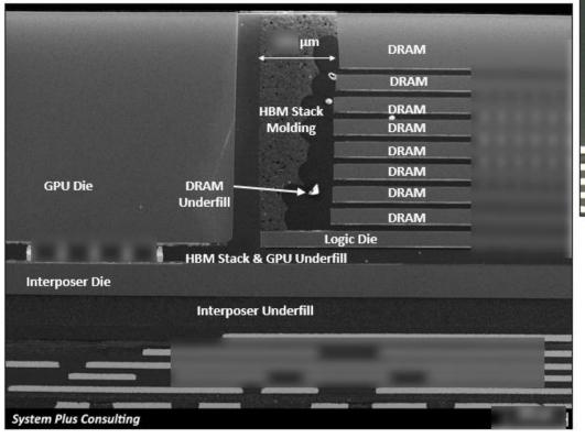
HBM Stack Cross-Section — SEM View
