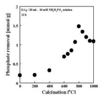
Figure 1. Phosphate removal on the product prepared at various calcination temperatures.
