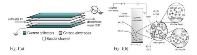
We show experimental and theoretical results of CDI in ion mixtures, where monovalent cations adsorbed early on, are later kicked out of the electrodes again by more slowly adsorbing divalent ions, resulting -after voltage reduction- in a water stream significantly enriched in divalent ions. This approach has potential for the selective desalination of water, the harvesting of valuable multivalent ions, and the selective removal of poisonous ions such as radionucleotides.
