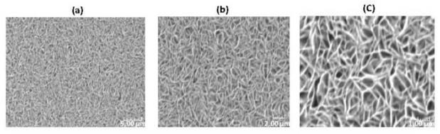
SEM pictures of birnessite thin films electrodeposited onto  $SnO_2$  (a) X 1000, (b) X 5000, (c) X 10000
