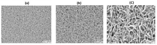
SEM pictures of birnessite thin films electrodeposited onto SnO2.
