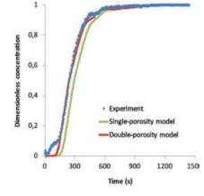
Figure 1. Solute transport in the porous medium before inoculation and after 17 days - Comparaison between experimental and numerical breakthrough curves at t=17 days
