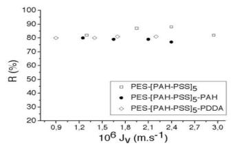
Copper retention rate (pH=2) as a function of the permeate flux for different PEM-modified membranes.
