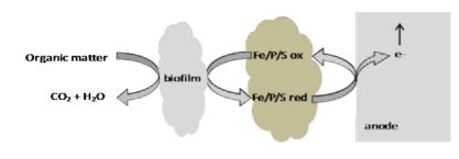
and power density features. The influences of anode parameters (surface, Fe/P/S composition, operating temperature...) were studied. A maximal power density of ~10 W.m<sup>-3</sup> at a current density of ~25 A/m<sup>3</sup> was obtained. Under these operating conditions, the treatment of 1 m<sup>3</sup> of 200 mg.L<sup>-1</sup> COD wastewater would
