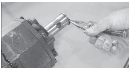
10. Remove PTO shaft snap-ring.
