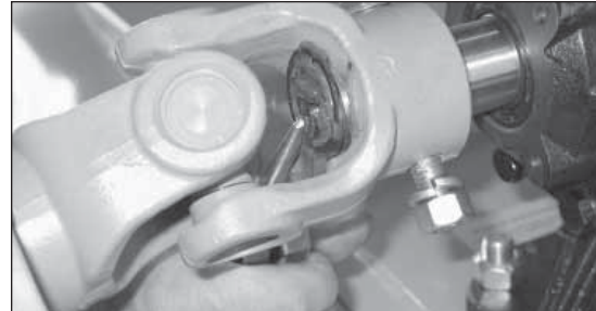
15. Reinstall snap ring on end of PTO shaft.
