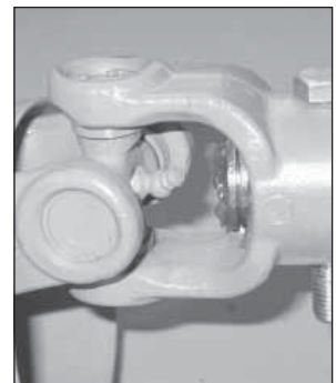
16. Grease two fittings on PTO shaft (one on each end of shaft in universal joint).
