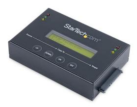
The SATDUP11IMG standalone SATA hard drive duplicator, lets you create an exact duplicate of a SATA hard drive (HDD) / solid state drive (SSD), or create a single backup library drive containing multiple images you can copy to additional drives at any time.
