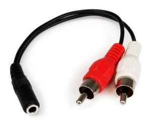
The MUFMRCA 6in 3.5mm to RCA stereo audio cable features one 3.5mm (TRS) female and 2x RCA male connectors, enabling you to connect your portable audio device ( iPod or other MP3 player) to your home stereo. Simply plug your audio device into the female 3.5mm connector using one of our standard male to male 3.5mm stereo audio cables (MU6MMS) and then connect to your home stereo through the two male RCA connectors.
