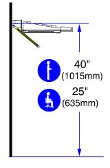
This mounting height is a recommendation for an ergonomic workstation. If user elbow heights are different than this, you should change mounting height to accommodate user elbow heights. (Change mounting height one inch for every one inch difference in user elbow heights).
