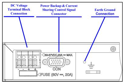
Figure 8-1: PD-90xxG Rear Panel Connectors
