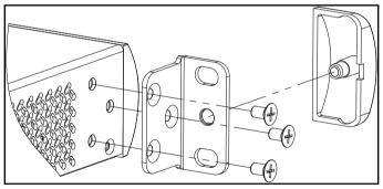
Figure 4-2: Installing Mounting Brackets
