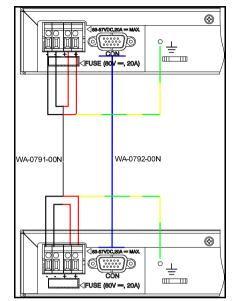
Figure 8-2: PD-90xxG Rear Panel connections
