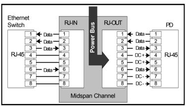
Figure 3-2: Connecting to Midspan
