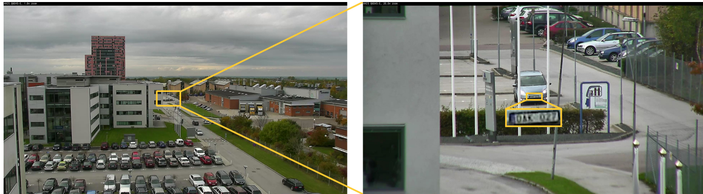
Snapshots of HDTV 1080p views from AXIS Q6045-E: at left, wide view; at right, 20x zoomed-in view where the license plate of a car 275 m (900 ft.) away can be read.
