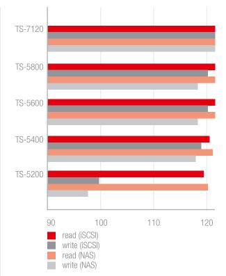
**Test environment:** N-Tec Rackmount Server Windows Server 2008R2, Dual XEON 32 GB RAM, 2 x IntelPRO/1000Dual = 4 x Gigabit NIC; Cisco SG300-10P 10 Port managed Gigabit with PoE.
