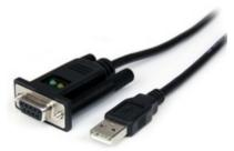
The ICUSB232FTN FTDI USB to Null Modem Serial Adapter Cable (1-Port) converts an available USB 1.1 or 2.0 port into an RS232 Null Modem serial DB9 port, solving DCE/DTE conflicts directly, without requiring additional cross-wired serial cables or adapters.
