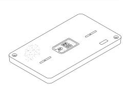
Available in cast iron for Quazite/FRP, plastic for PenCell
