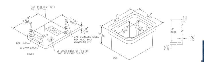
Covers DESCRIPTION TIER DESIGN / TEST LOAD # WEIGHT # PALLET QTY PART NO. W/2 Bolts 15 PC0608HA00\*\* 15,000 / 22,500 40 4 Gasketed w/4 bolts 15 40 PC0608HG00\*\* 15,000 / 22,500 4
