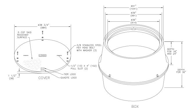
Covers DESCRIPTION TIER **DESIGN / TEST LOAD #** WEIGHT # PALLET QTY PART NO. W/ 3 Bolts PR3900CA00\*\* 8 8,000 / 12,000 141 10 (ዚ) W/ 3 Bolts 15 15,000 / 22,500 180 10 PR3900HA00\*\* (ዚ) W/3 Bolts 180 10 PR3900HH00\*\* 22 22,500 / 33,750
