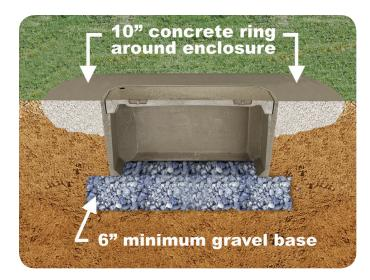
CONCRETE RING AROUND BOX 10 6 **QUAZITE® BOX & COVER** 6 COMPACTED EARTH **IN COMPACTED EARTH** ASPHALT PAVEMENT CONCRETE RING AROUND BOX **QUAZITE® BOX & COVER** 6 4 6 **IN ASPHALT PAVEMENTS** CONCRETE PAVEMENT D QUAZITE<sup>®</sup> BOX & COVER D D – 4 **IN CONCRETE PAVEMENTS**
