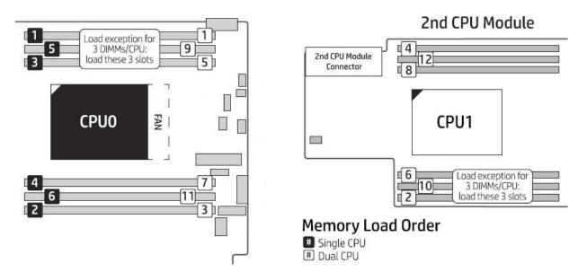
Maximum MemorySupports up to 768 GB DDR4-2933 ECC RAM\* (transfer rates up to 2933MT/s) and 384 GB DDR4-2666 ECC<br/>RAM (transfer rates up to 2666MT/s).
