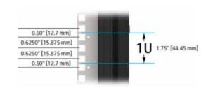
Figure 11. Rack mounting hole positioning in 1U rack space
