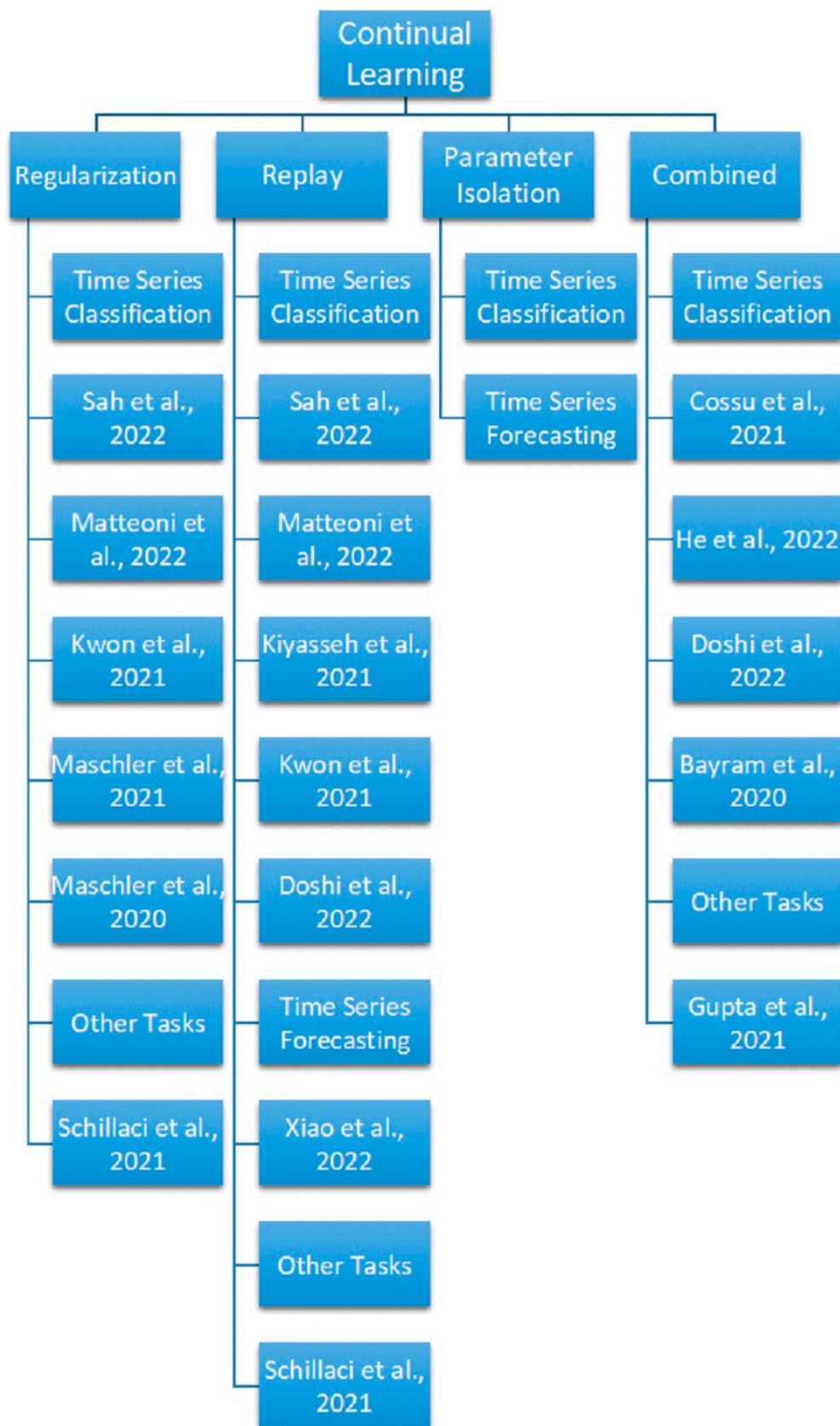
Figure 3. Tree diagram of the taxonomy of the continual learning methods for sensor time series classification and forecasting [93,94,106–116] (note: if a paper uses two methods separately with similar satisfactory results, the paper will be listed under both groups).
