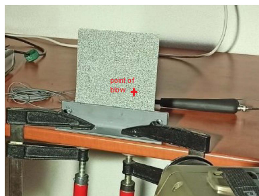
Figure 5. Laying of the analyzed steel plate and the excitation point.
