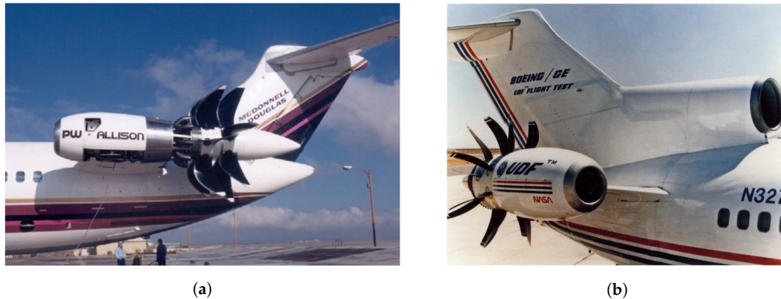
Figure 9. (a) Pratt & Whitney-Allison 578-DX geared propfan demonstrator engine, installed on an MD-80 testbed aircraft. (b) General Electric GE36 demonstrator engine installed on the Boeing 727 testbed for flight testing in 1986–1987.
