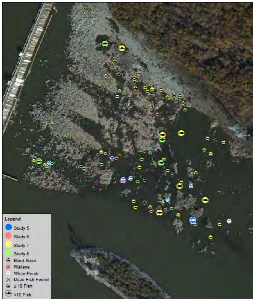
Figure 2 a & b. As documented in RSP 3.8 Figure 4.2-2-2, during the Summer, fish stranding and mortality was documented (a) in a portion of the channel that is dewatered between 86,000 cfs and 30,000 cfs (b). Downramping rates below 30,000 cfs would not be expected to mitigate these stranding and mortality impacts.
