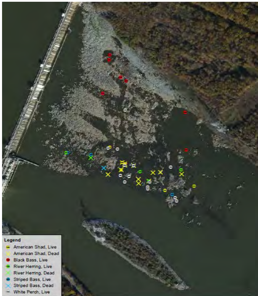
Figure 1 a & b. As documented in RSP 3.8 Figure 4.1-2-2, during the Spring, fish stranding and mortality was documented (a) in a portion of the channel that is dewatered during downramping between 86,000 cfs and 30,000 cfs (b). Downramping rates below 30,000 cfs would not be expected to mitigate these stranding and mortality impacts.
