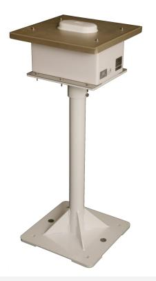
Mesotech's thunderstorm and lightning sensor detects electrical discharges associated with lightning within a 200 nautical mile radius of the system with a <2% false detection rate. This passive lightning detection sensor uses a receiving antenna to "listen" for electromagnetic signals.
