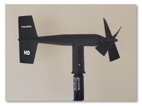
The mechanical wind sensor is high resolution and includes ice-resistant coating on external surfaces. The all-black color scheme enhances ice-shedding performance. The wind speed sensor is a four-blade helicoid-shaped propeller. Propeller rotation produces an AC sine wave with frequency directly proportional to speed. The AC signal is induced in a transducer coil by a six-pole magnet mounted on the propeller shaft. The coil resides on the non-rotating central portion of
