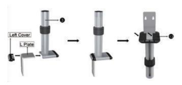
Desk Clamp: Attach the bottom portion of the Clamp (4) to the L Plate, then place
