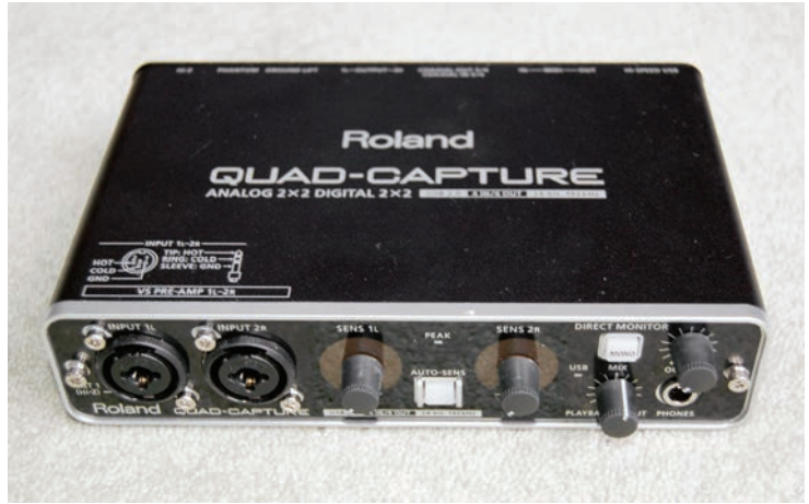
A Roland Quad-Capture. "It has fully variable analogue input level adjustment on each channel and proper level metering, unlike the Furutech GT40a", says David Lord.
