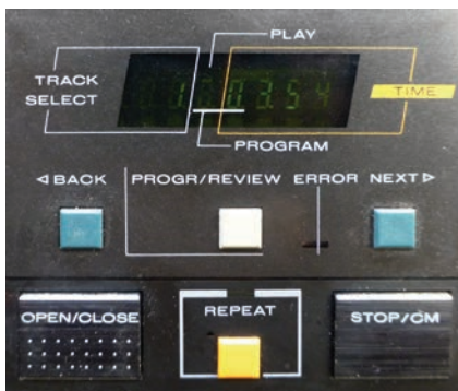
The CD104's diminutive display, and some of its 'no-nonsense' controls. To the right of these is a rectangular panel with the Play, Pause and Forward/Reverse search buttons.
