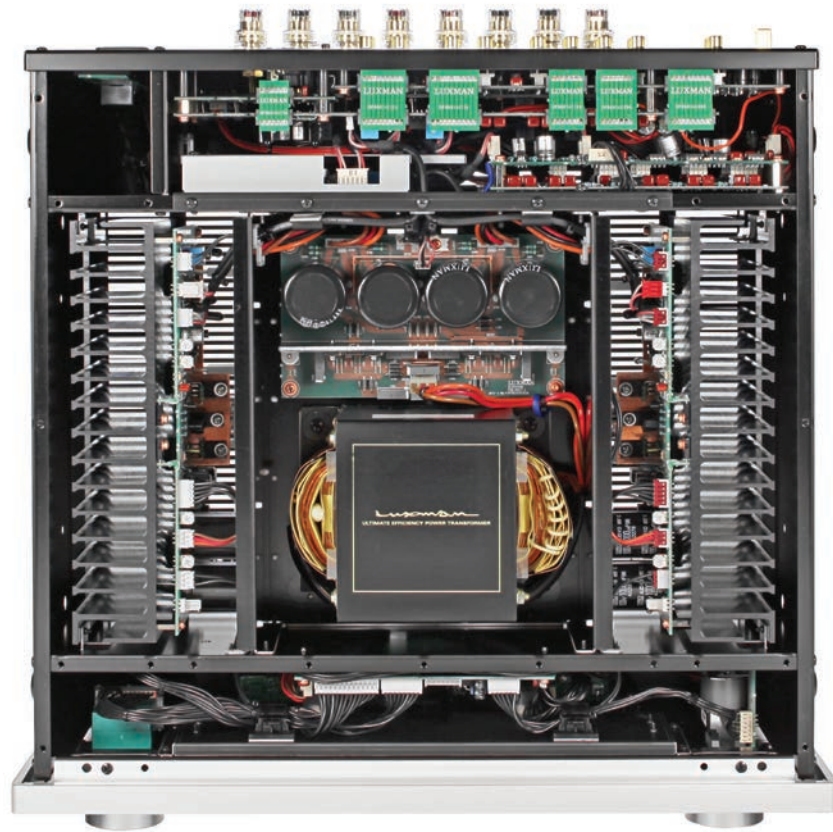
Internally the Luxman's block construction incorporates shielding panels to isolate the individual sections while oxygen-free copper cabling is used throughout. Big heatsinks absorb heat produced by Class A working, and at centre lies a big, linear power supply.
