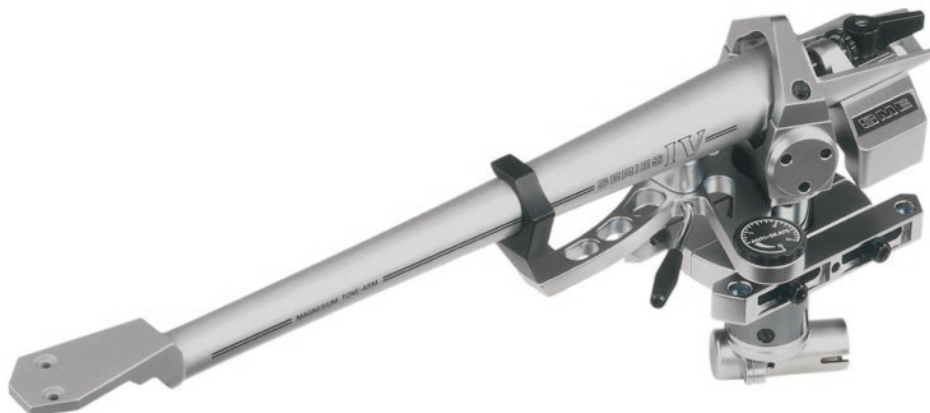
The SME IV arm used by David Lord. Its output socket at the base of the pillar delivers a balanced signal. To go balanced the connecting cable must be changed to a 3-pin XLR on each channel or one 5-pin type.
