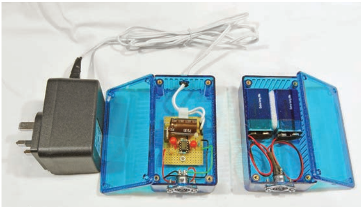
Fig 14. The power supplies: mains supply from a 24V a.c. wall wart at left, battery supply at right.
