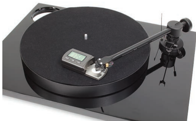
One "greatest audio landmark" for Jonathan Ledger was "spending a whole day setting up and realigning my tonearm and turntable". There's plenty to do, aligning the arm's geometry, assessing bias force and ensuring tracking force is ideal. Use a modern digital gauge, as above, to get this right.
