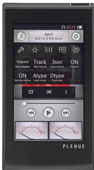
Yes – you even get output level meters on the Plenué I! They are a display option, with red bar graph meters an alternative. Note the small red volume level readout at top right, and low resolution battery indicator – both difficult to read.
