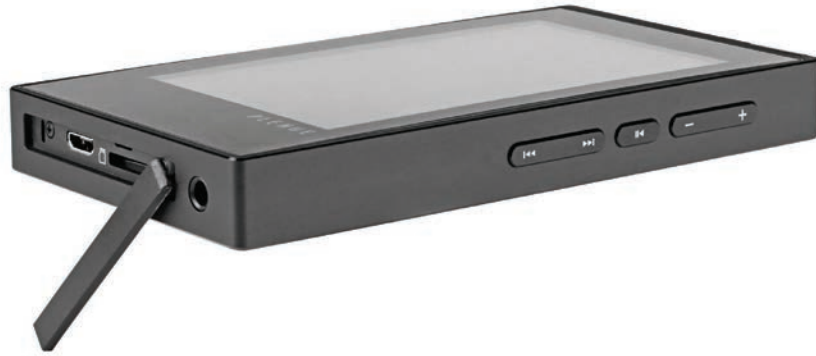
A small plastic captive clip-on cover protects the player's ports from pocket lint. A microSD card slot and microUSB port are visible here, plus the exposed 3.5mm headphone jack. This jack also houses an optical S/PDIF digital output. There's no volume control, just Up and Down buttons, also seen here.
