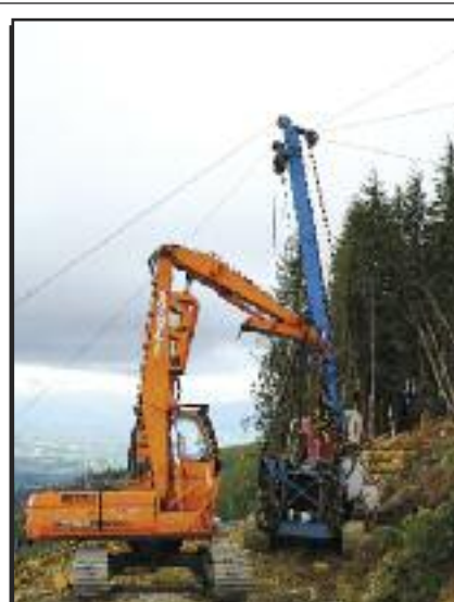
ON THE COVER: VanDyk and Son's Doosan 225 gets the processing done out on the job in NW Washington with the 45-foot TTY 45 yarder in the background. See "Bulls in the Woods" starting on Page 8
