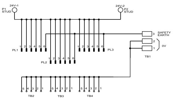
Figure 2 Trusted Output Power Distribution Unit – Wiring Diagram
