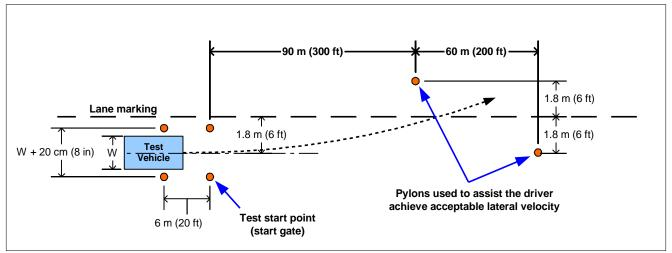
Figure 1. Position of Cones Used to Assist Driver
