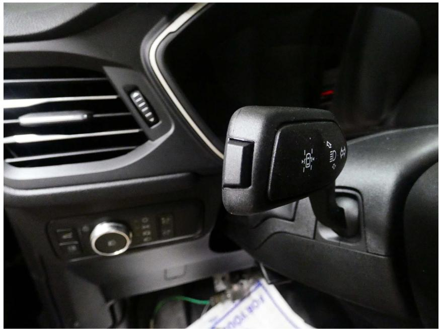
Figure A10. LDW System On/Off Button
