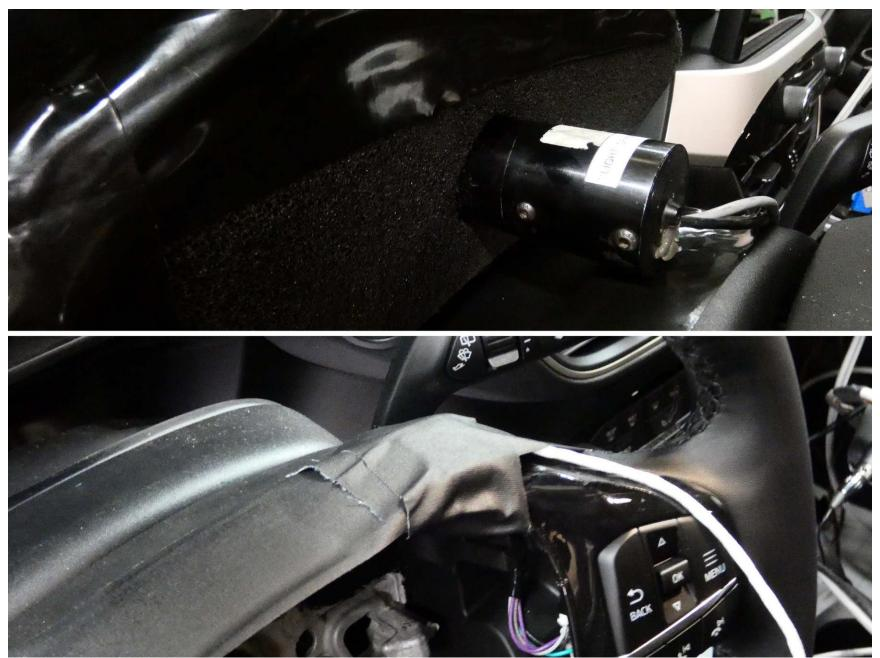
Figure A8. Sensors for Detecting Visual and Haptic Alert
