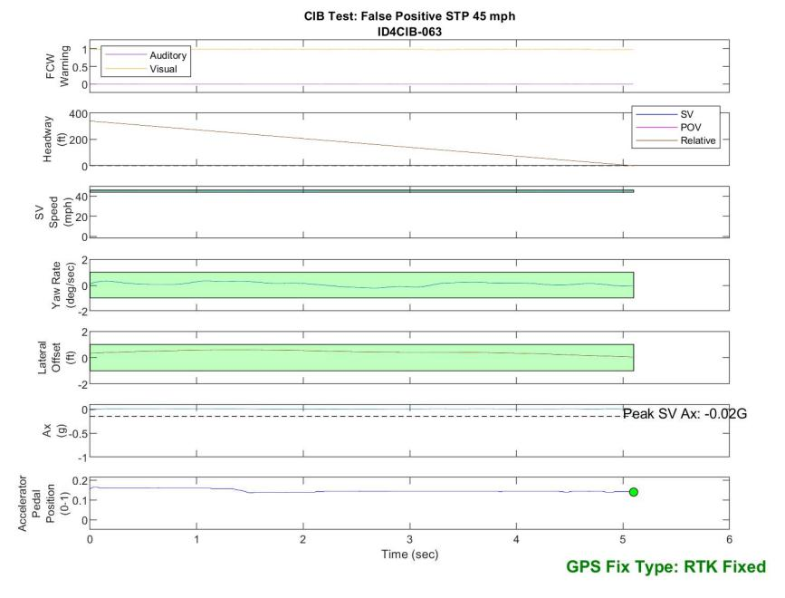
Figure D50. Time History for CIB Run 63, SV Encounters Steel Trench Plate, SV 45 mph
