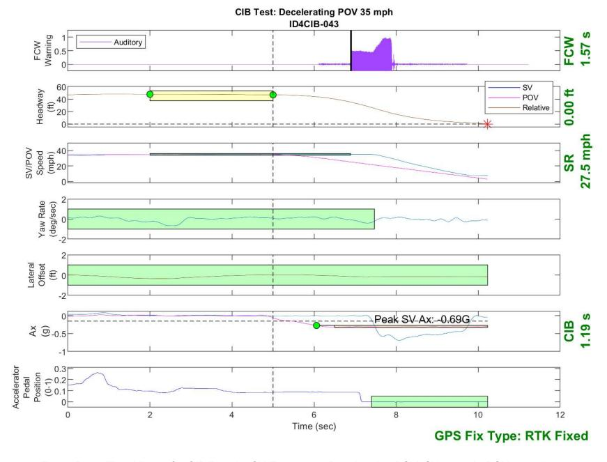
Figure D33. Time History for CIB Run 43, SV Encounters Decelerating POV, SV 35 mph, POV 35 mph
