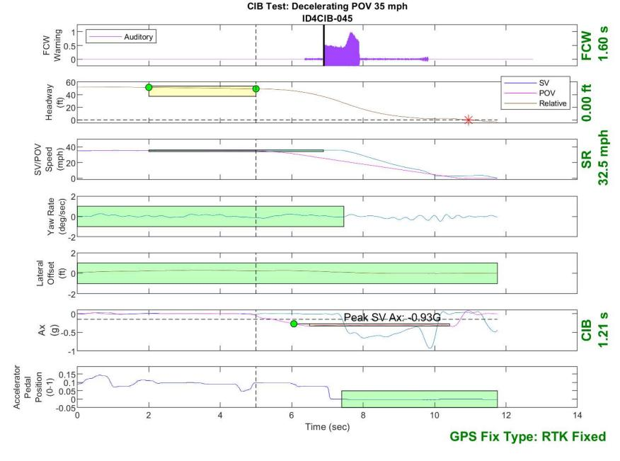
Figure D35. Time History for CIB Run 45, SV Encounters Decelerating POV, SV 35 mph, POV 35 mph
