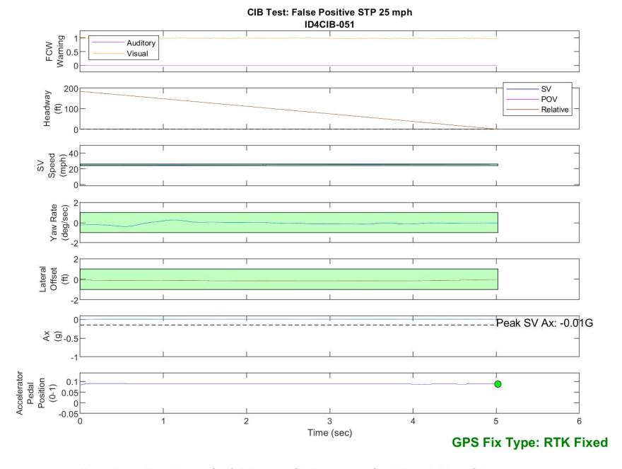
Figure D39. Time History for CIB Run 51, SV Encounters Steel Trench Plate, SV 25 mph
