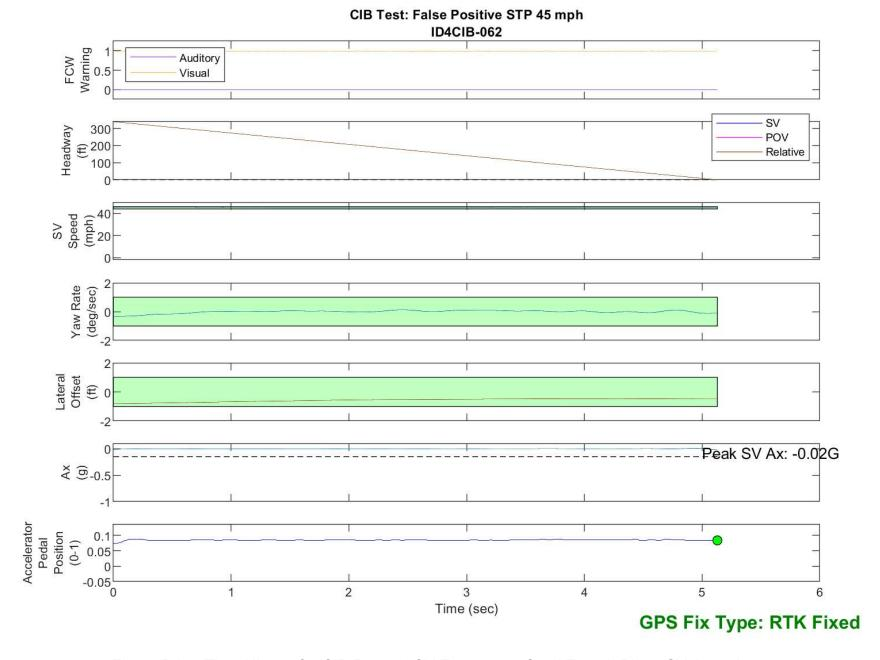
Figure D49. Time History for CIB Run 62, SV Encounters Steel Trench Plate, SV 45 mph
