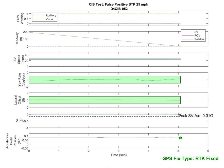
Figure D40. Time History for CIB Run 52, SV Encounters Steel Trench Plate, SV 25 mph
