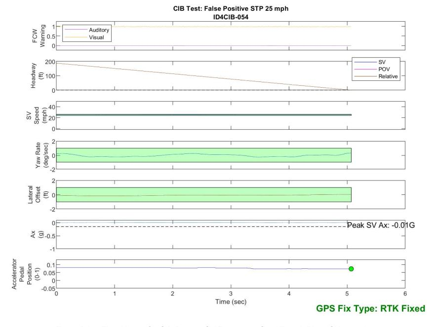
Figure D42. Time History for CIB Run 54, SV Encounters Steel Trench Plate, SV 25 mph
