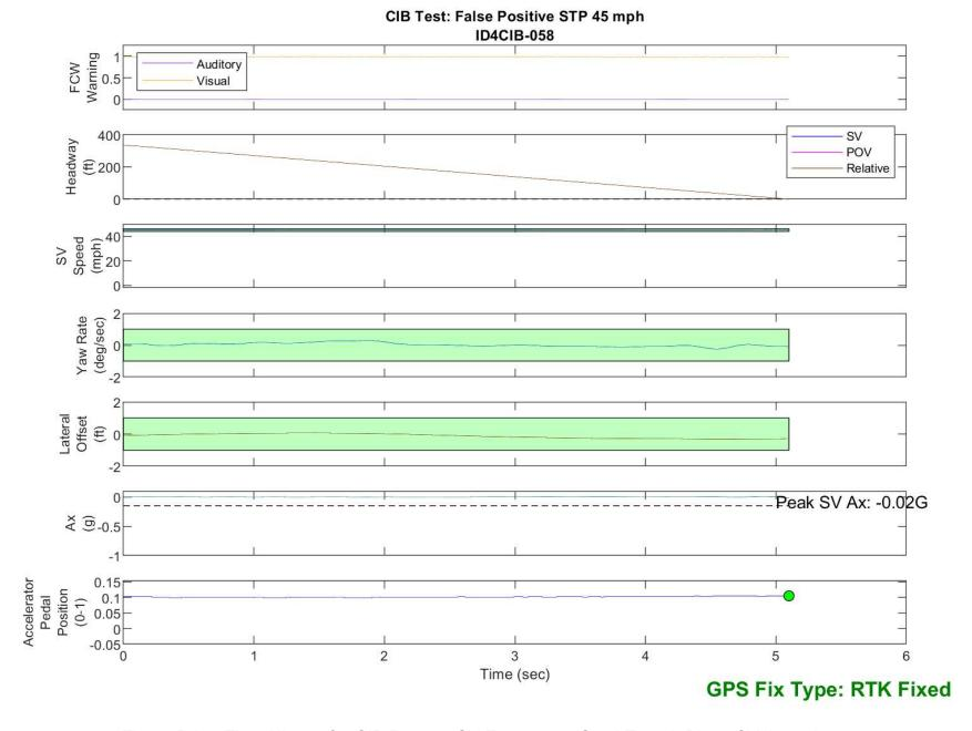
Figure D45. Time History for CIB Run 58, SV Encounters Steel Trench Plate, SV 45 mph
