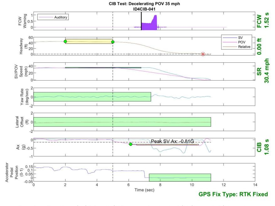
Figure D32. Time History for CIB Run 41, SV Encounters Decelerating POV, SV 35 mph, POV 35 mph
