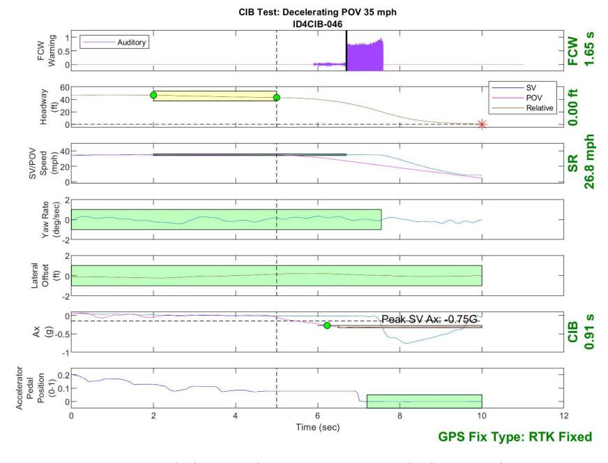
Figure D36. Time History for CIB Run 46, SV Encounters Decelerating POV, SV 35 mph, POV 35 mph
