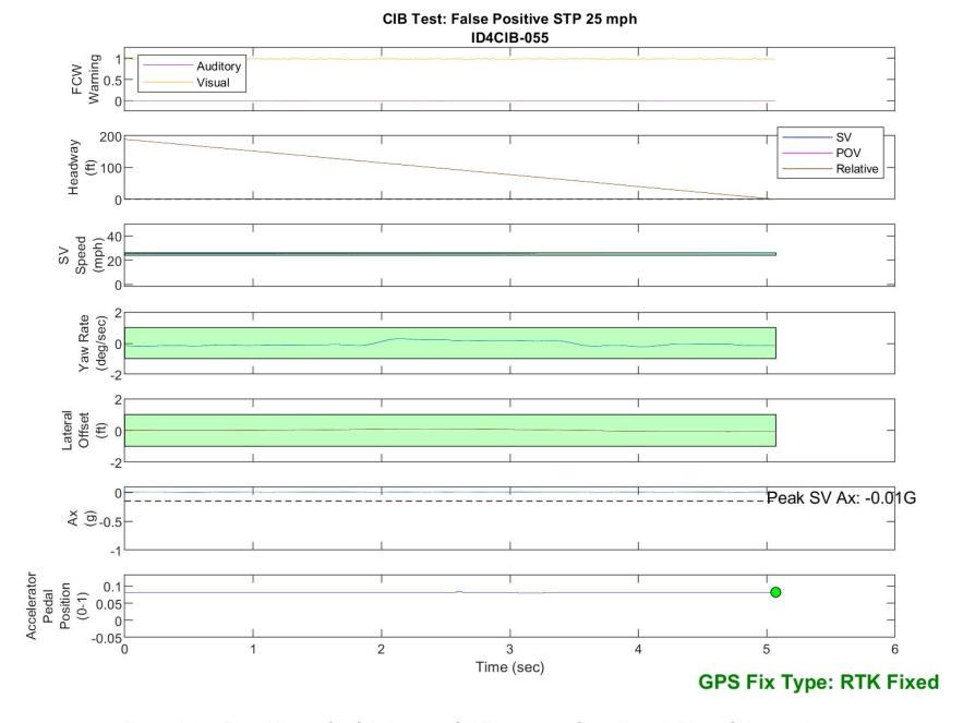
Figure D43. Time History for CIB Run 55, SV Encounters Steel Trench Plate, SV 25 mph
