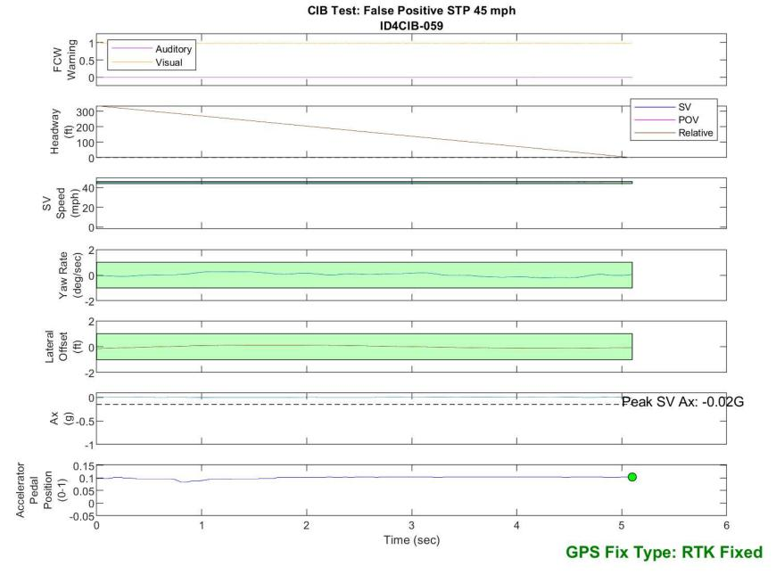
Figure D46. Time History for CIB Run 59, SV Encounters Steel Trench Plate, SV 45 mph
