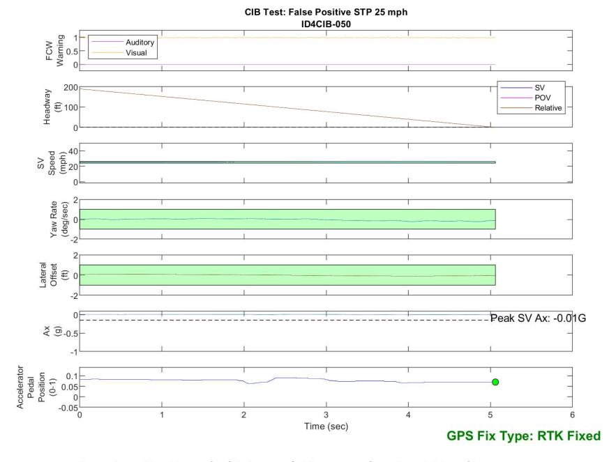
Figure D38. Time History for CIB Run 50, SV Encounters Steel Trench Plate, SV 25 mph
