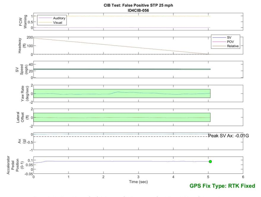
Figure D44. Time History for CIB Run 56, SV Encounters Steel Trench Plate, SV 25 mph
