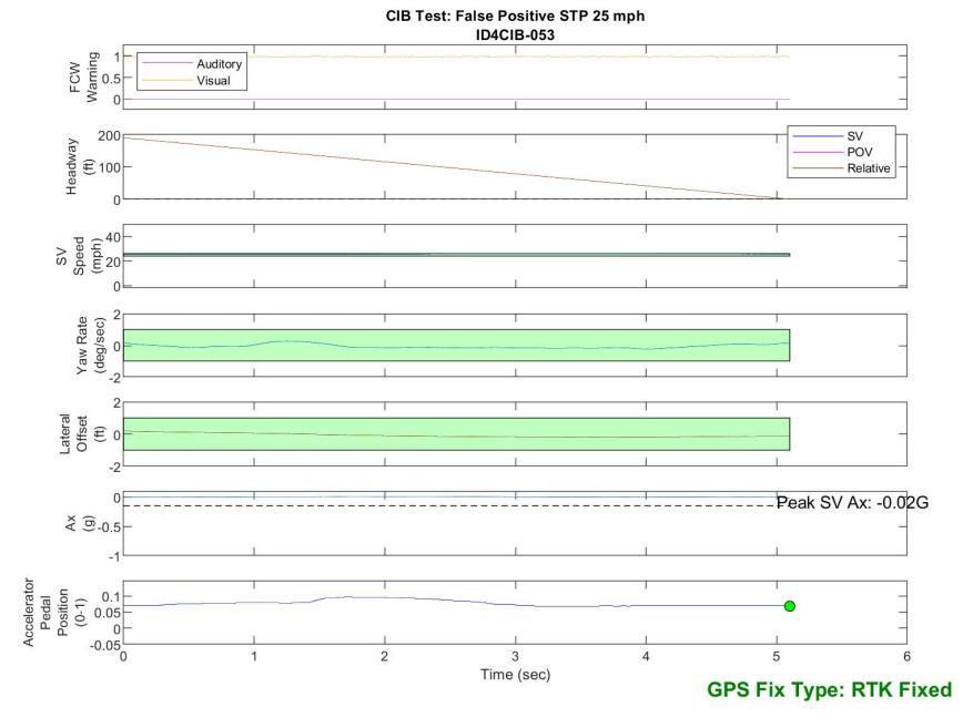
Figure D41. Time History for CIB Run 53, SV Encounters Steel Trench Plate, SV 25 mph
