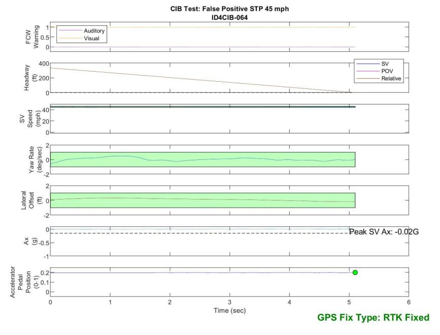
Figure D51. Time History for CIB Run 64, SV Encounters Steel Trench Plate, SV 45 mph
