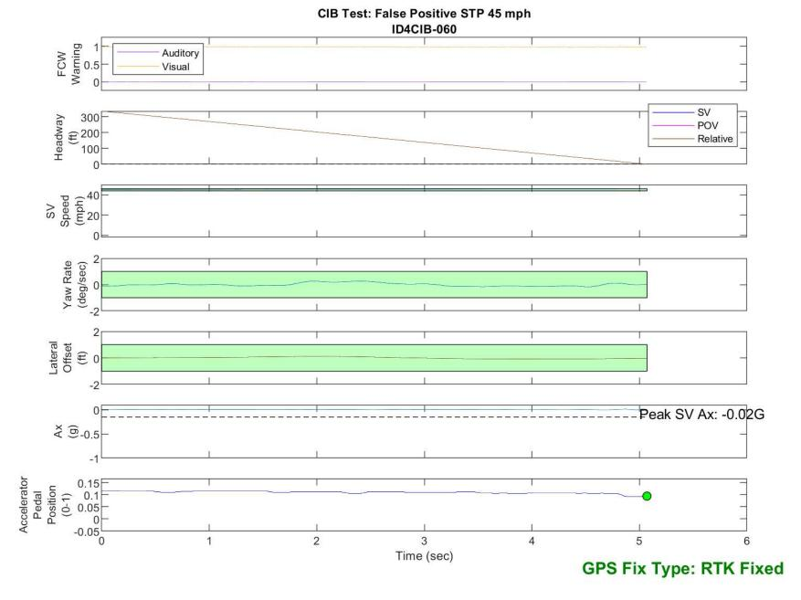
Figure D47. Time History for CIB Run 60, SV Encounters Steel Trench Plate, SV 45 mph
