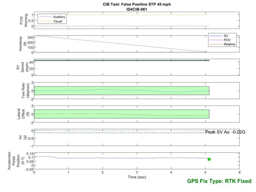
Figure D48. Time History for CIB Run 61, SV Encounters Steel Trench Plate, SV 45 mph
