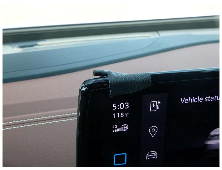
Figure A11. Sensor for Detecting Auditory Alert
