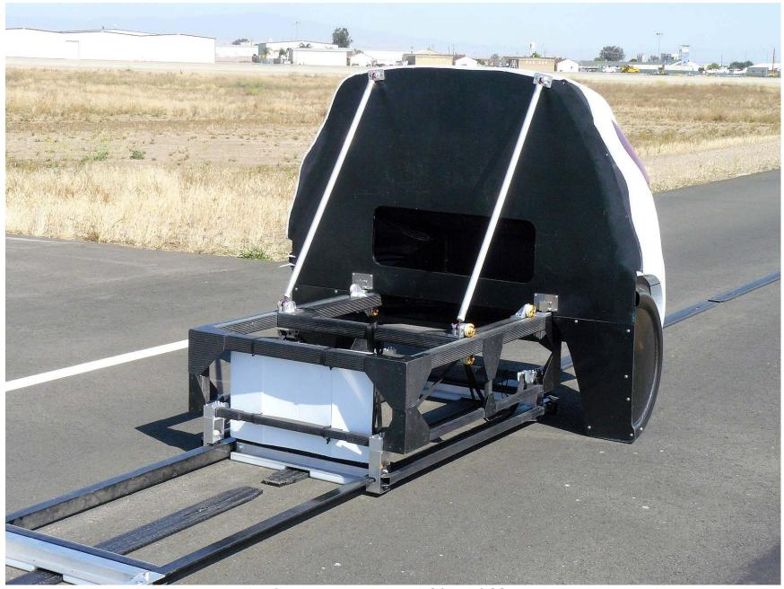
Figure A7. Load Frame/Slider of SSV
