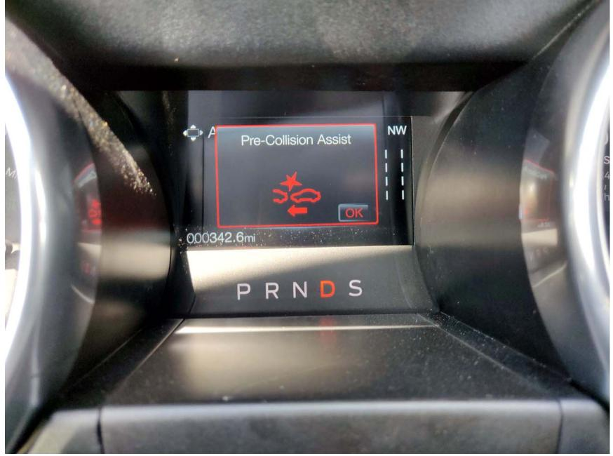
Figure A16. Instrument Panel AEB Visual Alert
