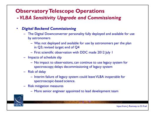
The goal of the DDC FPGA personality is to provide flexible spectroscopic observing modes using the VLBA's digital backends. The complexity of the design has made it difficult to implement, and in FY12 Q2 it was found that aliased out-of-band signals (and noise) were affecting the bottom ~6 MHz of each sub-band, preventing the DDC from being useful for narrowband spectroscopy. While this problem is being addressed the legacy backends are continuing to be used for spectroscopic observations.
