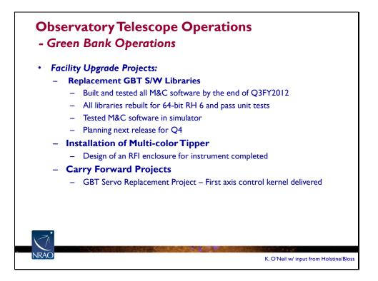
**Replacement GBT S/W Libraries** – The Software Division built and tested all M&C software in Q3. All libraries were rebuilt for 64-bit Red Hat v6 and passed unit tests. M&C software tested in simulator. Planning next release for Q4.
