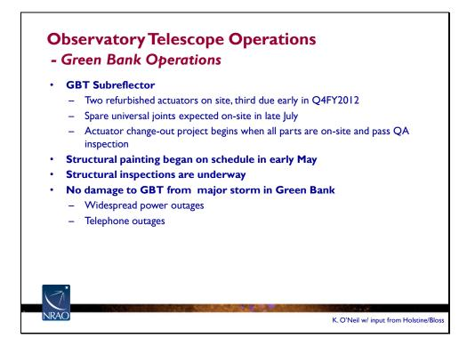
Work continues on refurbishment of the **subreflector actuators** following mechanical failure of the X2 actuator last fall and the Y2 actuator in March. X2 and the spare Z unit have been refurbished and are back on site; Y2 is nearly finished at the manufacturer. Spare universal joints are in fabrication and delivery is expected by the end of July. Changeouts of the other units will begin using these units after that.
