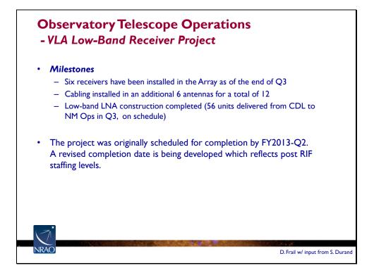
VLA low-band receivers: Six receivers were install in the array. It is anticipated that 6 additional receivers will be installed by the end of FYQ4 for a total of 12 receivers. Performance of the system 4-band (50-80 MHz) Trx = ~401 degrees K, P-band (230 - 470 MHz) Trx = ~66 degrees K.
