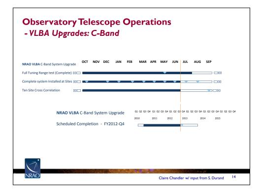
NL, BR, and MK were outfitted with complete C-band systems during Q3, to provide 8 complete systems, ahead of schedule.
