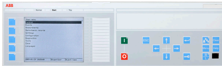
Figure 17: Local human-machine interface
